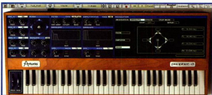
FIG. 1: The Mixer section of the Envelopes tab has a 5-segment envelope for automating the vector in Arturia Prophet-V.
