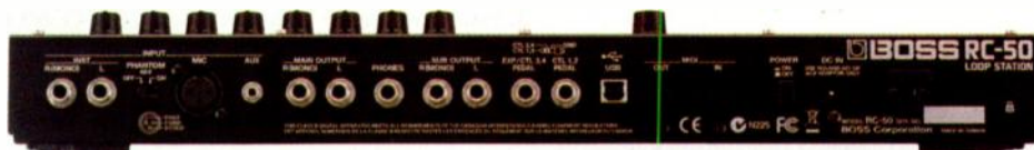
FIG. 2: On the RC-50's rear panel are two ¼-inch inputs, an XLR input with phantom power, a stereo minijack input, two ¼-inch main outputs, a stereo headphone output, two ¼-inch sub outputs, two foot controller inputs, a USB port, MIDI In and Out, a power switch, and a wall-wart connection.
