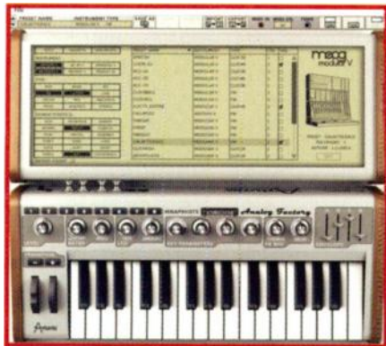
Analog Factory's control panel shows the Preset Manager on top, with the keyboard and synth controls on the bottom. You can hide either view.
