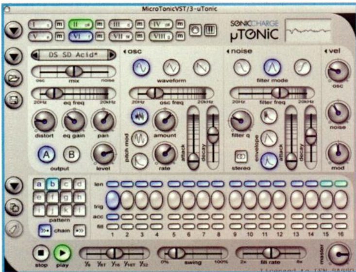
FIG. 11: MicroTonic is a classic synthesized drum machine featuring a 12-pattern 16-step pattern sequencer to play its oscillator and noise sound generators.
