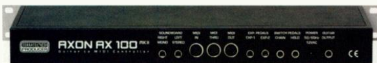
FIG. 2: The Axon AX 100 mkII's rear panel houses all of its audio, MIDI, footswitch, and pedal connections.
