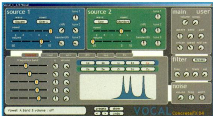
FIG. 1: You use Vocal's formant-filter editor to construct two sets of five formants.
