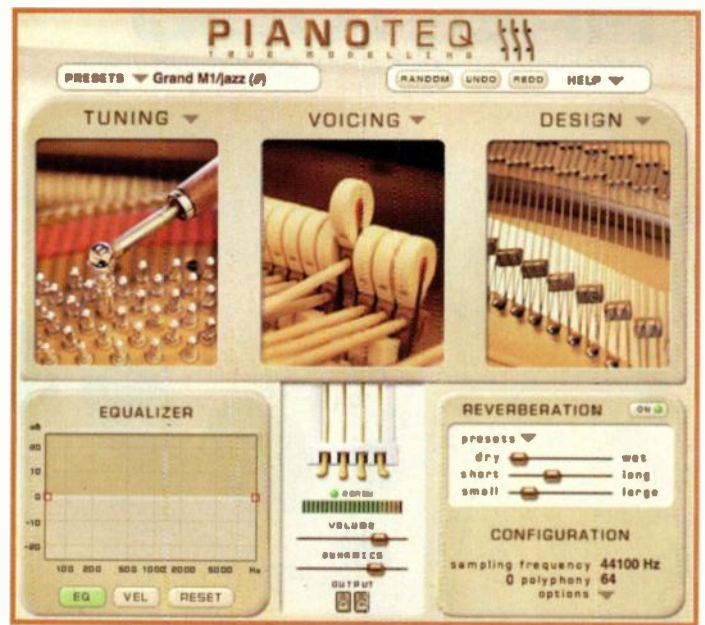
FIG. 1: Pianoteq's control panel is laid out in three horizontal sections: preset management and help (top), physical-modeling panels (middle), and pedals and playback controls (bottom).
