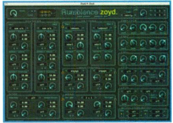
FIG. 12: Zoyd's two oscillators are followed by filters, waveshapers, and a mixer whose signal routing can be reconfigured.
