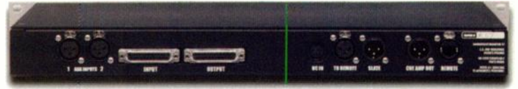
FIG. 2: In order to fit all of the I/O capabilities onto the back panel of the Monitor ST, D-sub connectors were used for the main inputs and outputs.
