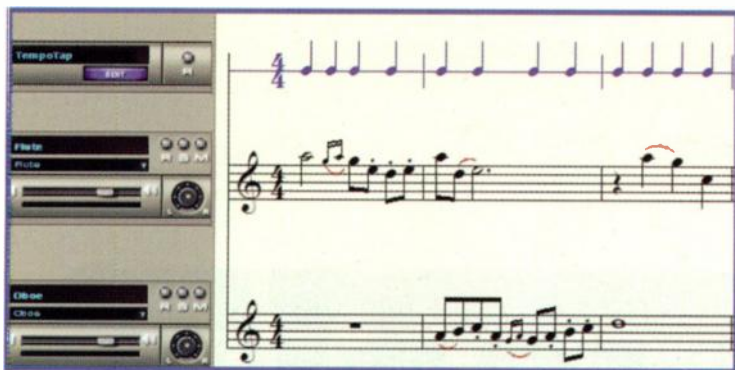
FIG. 3: Studio view combines traditional music notation with faders and panners reminiscent of a sequencer. The top staff is used with the TempoTap feature that lets you conduct tempo changes by tapping a MIDI or QWERTY key.
