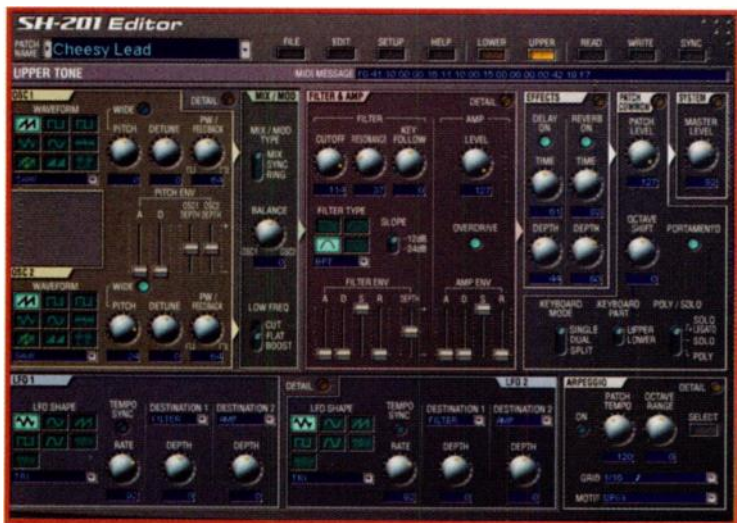
FIG. 2: The included software editor for the SH-201 provides access to a number of parameters not available from the instrument's front panel. Its amenities include a MIDI Message data field (upper right), which shows the System Exclusive or Control Change message being sent for each edit. These messages can be copied and pasted into your sequencer.
