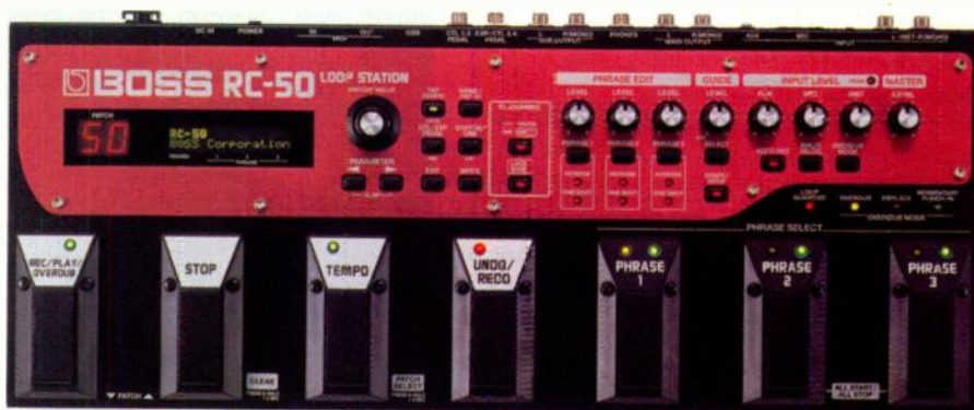
FIG. 1: The Boss RC-50 is a real-time audio looper housed in a floor processor with seven footswitches, plenty of hands-on controls, and 24 minutes of stereo recording time.
