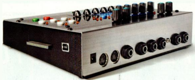
FIG. 2: The back of the 2880 houses all of the input and output connections except for the USB connector and the CompactFlash card slot, which are on the right side.
