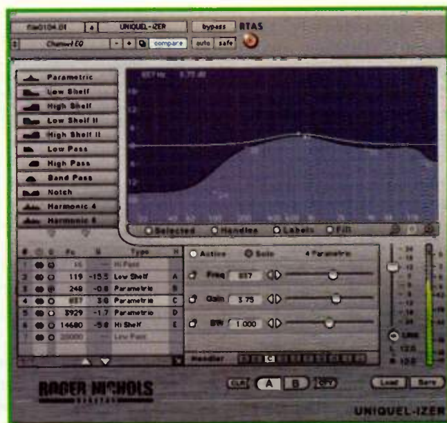
FIG. 1: Uniquel-izer gives you control over how many bands and what types of filters you want to use.
