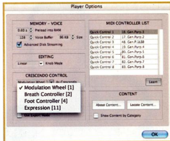
FIG. 2: Clicking on the Options button opens a dialog box in which you can assign MIDI controllers and make adjustments that affect HSO's demands on your computer.
