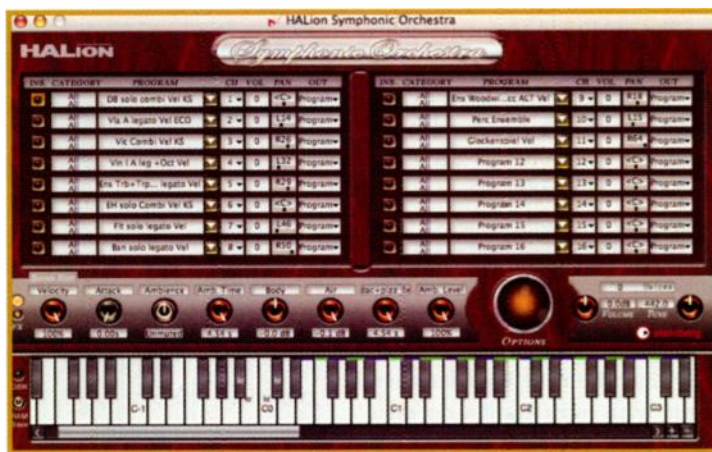
FIG. 1: Like other software built on the HALion Player platform, HALion Symphonic Orchestra is 16-part multitimbral and allows you to route each part to individual stereo outputs.
