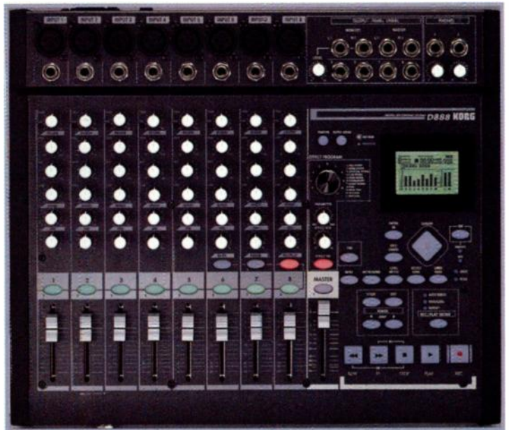
FIG. 1: Korg's D888 is a capable digital mixer and recorder intended for live use. It combines eight XLR and eight balanced/unbalanced TRS inputs with 3-band EQ per channel strip and a 40 GB internal hard drive.
