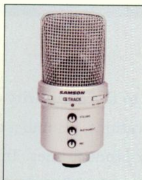
FIG. A: The Samson G-Track can also be used as a 2-channel interface.
