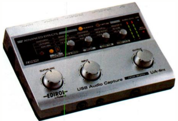
The UA-4FX's top panel sports the effects selector; four effects parameter knobs; and large input, output, and guitar/mic input-level knobs. I/O jacks and mod switches line the front, rear, and side panels.
