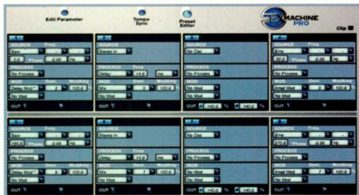
FIG. 1: In the glitchless pitch-shifter, the top and bottom rows of modules render the same time-stretching process with a 180-degree phase shift.
