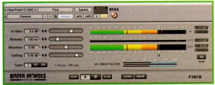
FIG. 4: Finis is a brickwall limiter that features the Crest Factor Meter, which lets you easily gauge the effect of the limiter on your material's dynamic range.
