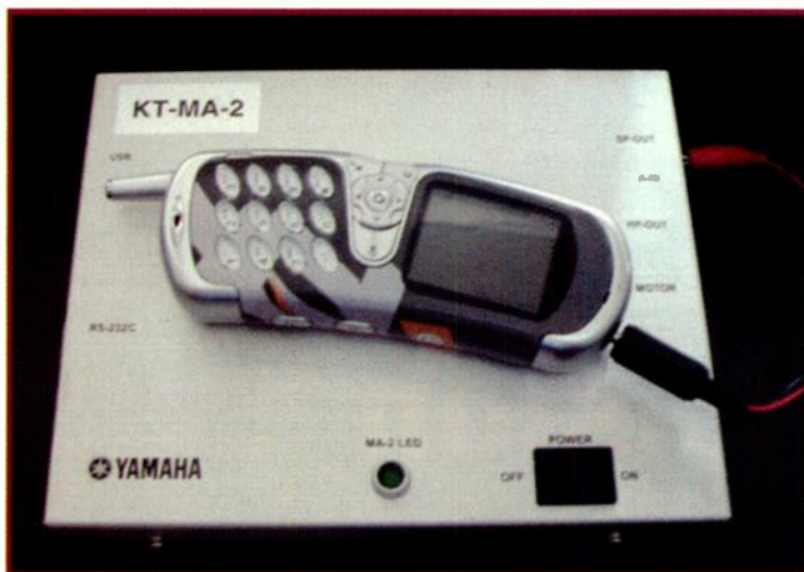
FIG. 3: Shown here are some tools of the trade: a Yamaha MA2 developer box with a dummy phone connected to audition the sounds.
