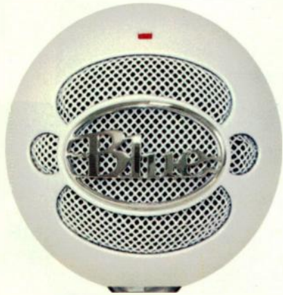
FIG. 2: The Blue Microphones Snowball offers omnidirectional and cardioid polar patterns, as well as a cardioid setting with a -10 dB pad.
