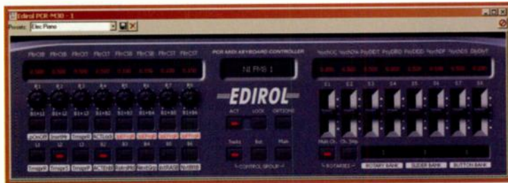
FIG. 2: Sonar's Active Controller Technology provides excellent support for Ediol PCR controllers. Also available is a generic ACT surface that supports many common controllers.
