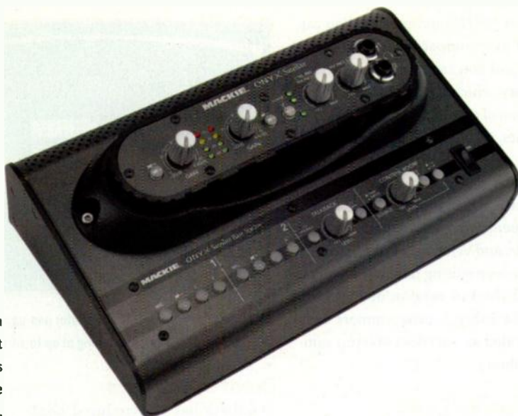
FIG. 1: The Onyx Satellite is a FireWire audio interface that hosts a preamp pod, which is removable for use in remote recording sessions.
