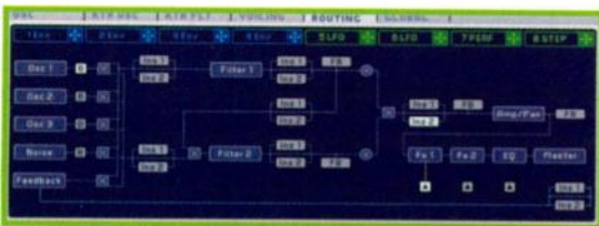
FIG. 2: You can reconfigure Massive's signal path by clicking on the icons in the Routing tab of the Central window.
