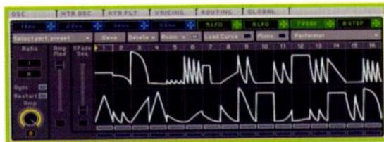
FIG. 4: Massive's Performance sequencer uses shapes as modulation sources at each step in the sequence.
