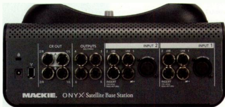
FIG. 2: On the base station, channels 1 and 2 each provide two line-level inputs, an instrument input, an XLR input, and an insert jack. Eight TRS output connectors allow you to set up a surround mix in your audio software.
