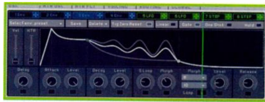
FIG. 3: The sustain stage of Massive's envelopes allows you to morph between pairs of preset shapes and loop the chosen shape a fixed or unlimited number of times.
