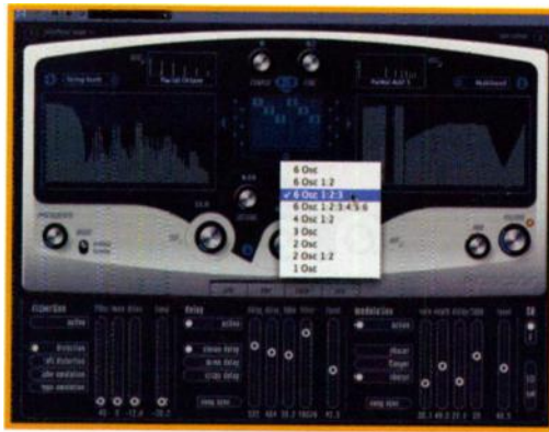
FIG. 3: You use Spector's Oscillator pop-up menu to set the relative tuning of up to six oscillator pairs.
