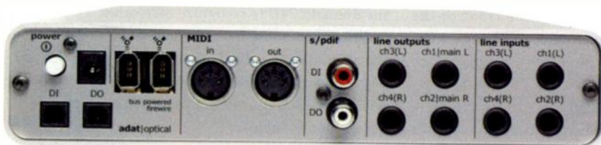
FIG. 2: Other than the front-panel combo jacks and the headphone outputs, the Konnekt 24D's I/O is all located on its rear panel.
