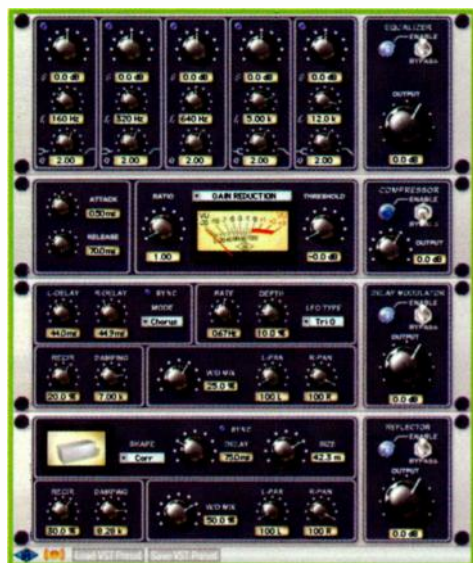
FIG. 2: CS-1 packs four processors into a single plug-in that provides EQ, compression, delay, and room simulation.
