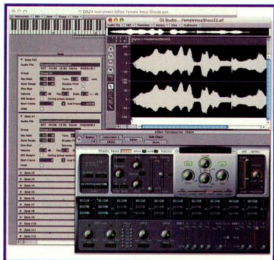
FIG. 2: In addition to its main interface, Apple EXS24 mkII furnishes Sample and Instrument Editor windows for creating and modifying multisampled instruments.
