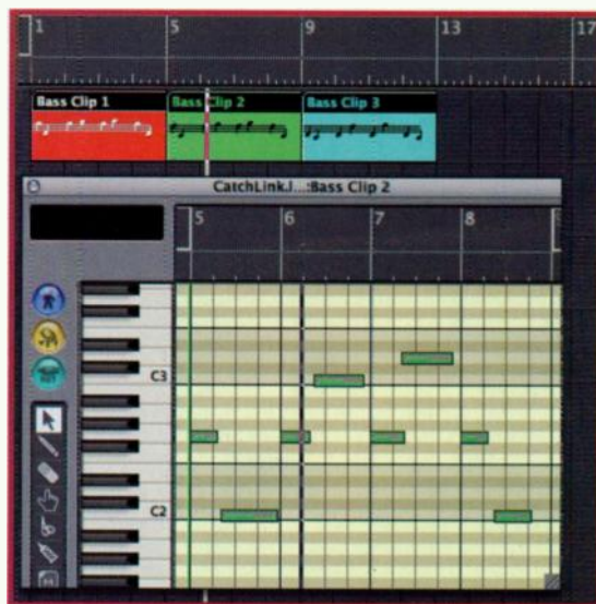
FIG. 2: In Contents Catch mode, the Matrix Edit window reveals the contents of the MIDI region currently being played.
