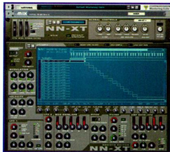
FIG. 8: One of two samplers in Propellerhead Reason, NN-XT lets you map samples, apply filtering, and route modulators in its Remote Editor window.
