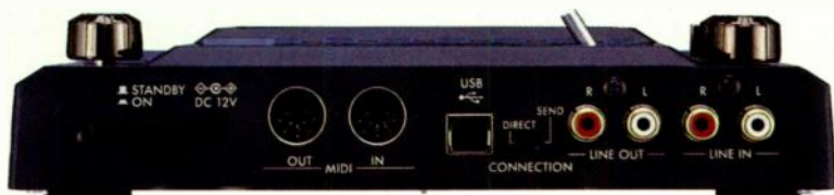
FIG. 2: The KP3's back panel includes a power jack (with no cord lock), MIDI I/O, USB, a Direct/Send switch for in-line or aux-send hookups, and RCA audio I/O. A headphone output, a 1/4-inch mono mic input, and an SD card slot are on the front.
