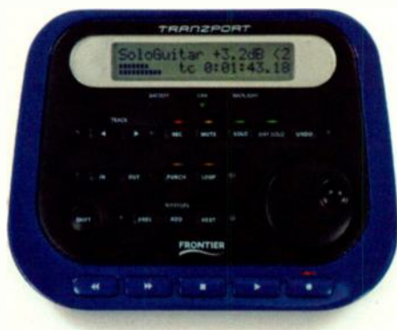
FIG. 1: The Frontier Design Group TranzPort wireless DAW controller is excellent for working from an alternate position in the control room.
