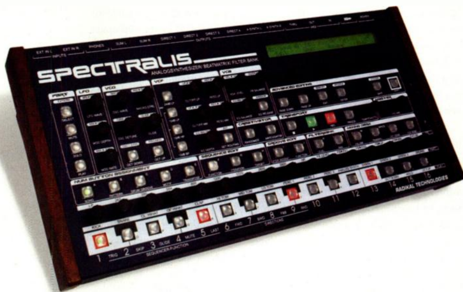
FIG. 1: The Spectralis is more than a synth module with sample-playback and virtual analog sound engines. It's also a sophisticated drum machine, step and pattern sequencer, and 10-band filter bank.
