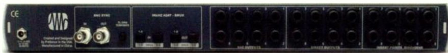
FIG. 2: A multitude of analog outputs, including preconverter insert points, makes the DigiMax FS a serious front end for studios with ADAT Lightpipe connections.
