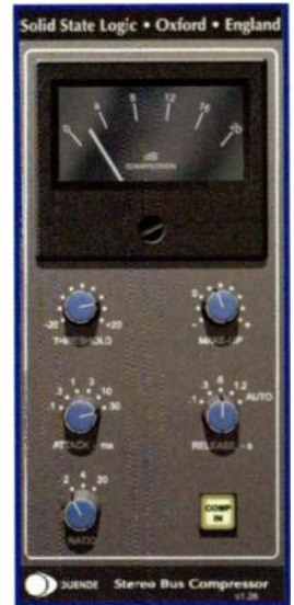
FIG. 2: Bus Compressor is modeled on the 4000 console's master bus compressor, famed for its ability to pull together mix elements.
