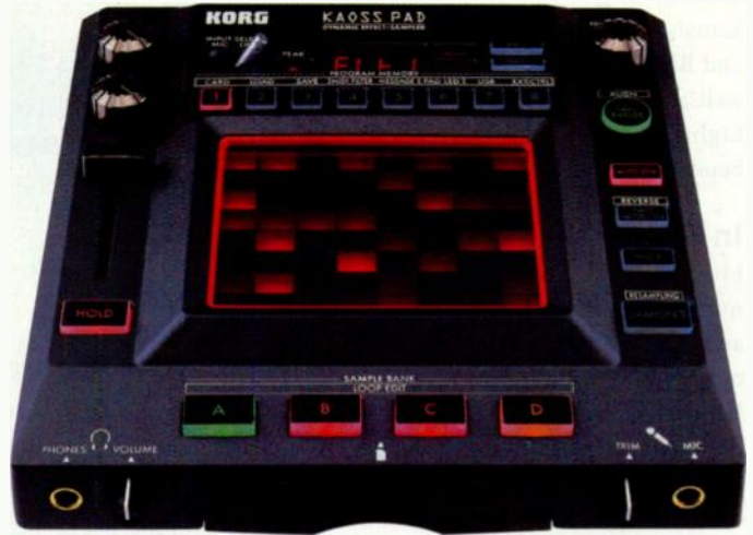
FIG. 1: Play your effects (or your soft synths) with the KP3's 8 × 8 light-up display. A trail of LEDs follows your finger to show the last value. The four sample pads trigger one-shots and unmute loops.
