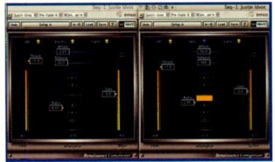
FIG. 8: A lead vocal track is compressed by two Waves Renaissance Compressor plug-ins chained in series.
