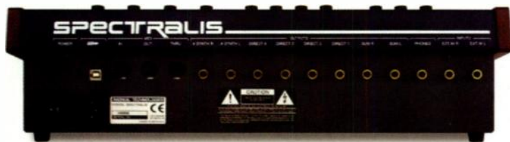
FIG. 2: In addition to MIDI and USB ports, the Spectralis has nine analog audio outputs and a pair of audio inputs for processing external sounds through its filter bank.
