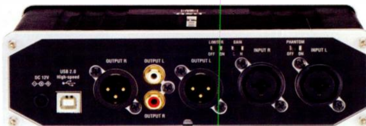
FIG. 3: On the MR-1000's rear panel, you'll find connections for analog audio I/O, USB 2.0, and 12 VDC power, as well as switches for phantom power, a limiter, and high or low gain.
