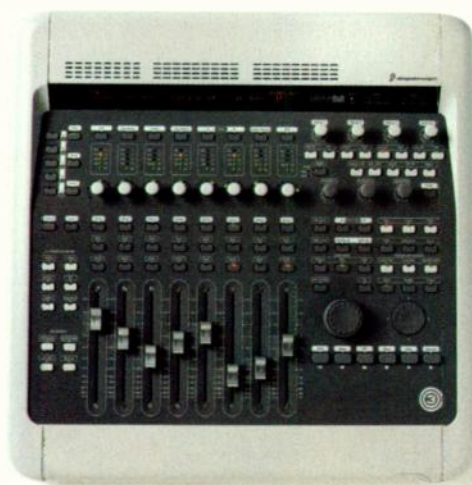
FIG. 1: The 003's control surface includes a jog/shuttle wheel and dedicated automation-mode buttons (middle left).
