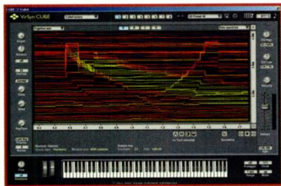
FIG. 2: The spectrum editor in VirSyn Cube 2 provides graphic tools with which you can warp the spectrum. Each horizontal line represents a different sine wave partial.
