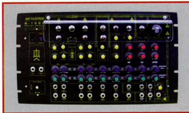
FIG. 2: Eleven unusual vacuum tubes are at the heart of the Metasonix Wretch Machine, a monophonic synth for people who like to take chances.
