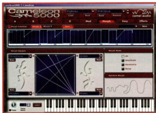
FIG. 1: An additive-based software synth might provide a two-dimensional vector envelope, such as this one in Camel Audio Cameleon 5000. The envelope is used to morph among four separate additive spectra.
