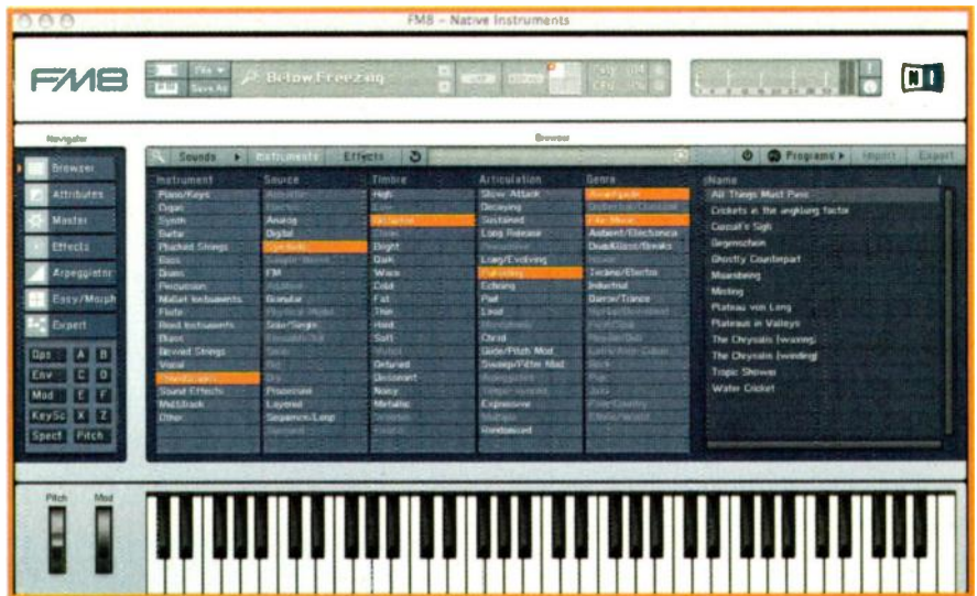
FIG. 1: One of FM8's two Browser interfaces. You select attributes and see matching patches, or view patches with a file-tree display.
