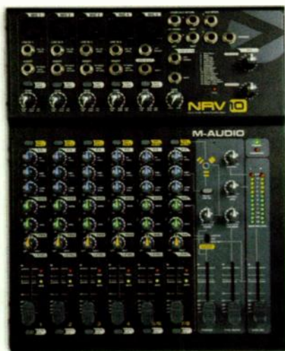
FIG. 3: M-Audio's NRV10 approaches the flexibility of full 2-way digital mixing by sending its channels to individual tracks of your computer audio application and routing the returns of those tracks back to individual channels of the mixer.
