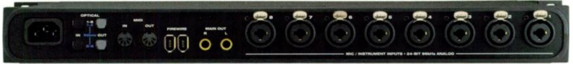
FIG. 2: The 8pre's rear panel includes four optical ports for high-resolution digital connections and two FireWire ports for connecting to a computer and daisy-chaining other FireWire devices.
