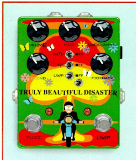
FIG. 3: The effects send and feedback loop in the Effector 13 Truly Beautiful Disaster can be controlled with the built-in photosensitive eye.
