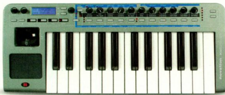
FIG. 1: Combining analog-modeling synthesis, a computer audio interface, and dozens of MIDI controllers, the Novation XioSynth 25 is a terrific value.
