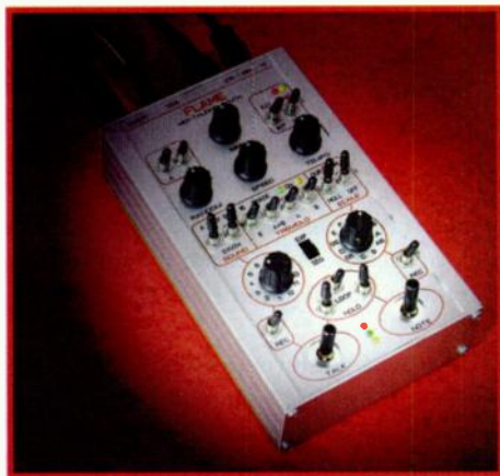
FIG. 1: The Rec, Loop, and Hold switches on the Flame MIDI-Talking-Synth let you set up repeating patterns.
