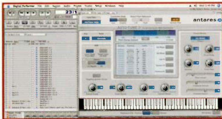
FIG. 1: Auto-Tune 5's Learn Scale From MIDI function. In this example, all diatonic notes for the scale of A minor are selected along with an F# (by inputting MIDI notes) to accommodate a song's temporary modulation into the key of G major. Note the I/O assignments for the record-enabled MIDI track (shown in Digital Performer's Track Overview window on the left) that feeds Auto-Tune.
