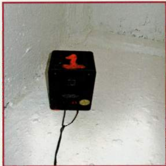
FIG. 2: Place a speaker near and facing into a corner of your echo chamber and adjust its position to get the sound you want.
