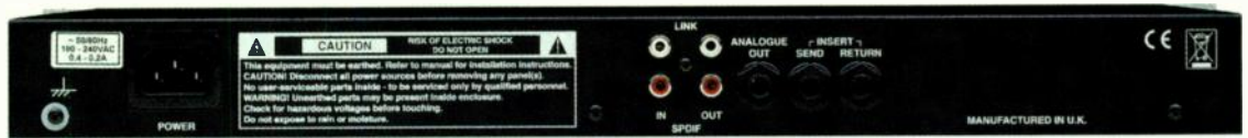
FIG. 2: The Alpha Channel's rear panel is basic, with analog audio and S/PDIF I/O and links to daisy-chain additional Alpha Channels.
