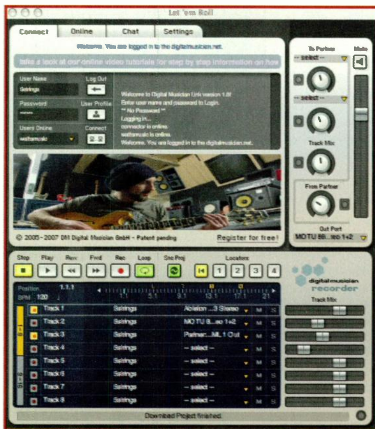
FIG. 1: digitalmusician.net's standalone DMR application is a multitrack recorder that lets you log in to a session without your browser. You can also use it as a ReWire app in conjunction with your favorite digital audio sequencer.
