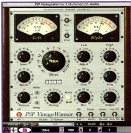
FIG. 3: Automap Universal wrapped plug-ins have a control bar added to the bottom of their GUI. You use that to create and edit settings on the fly.
