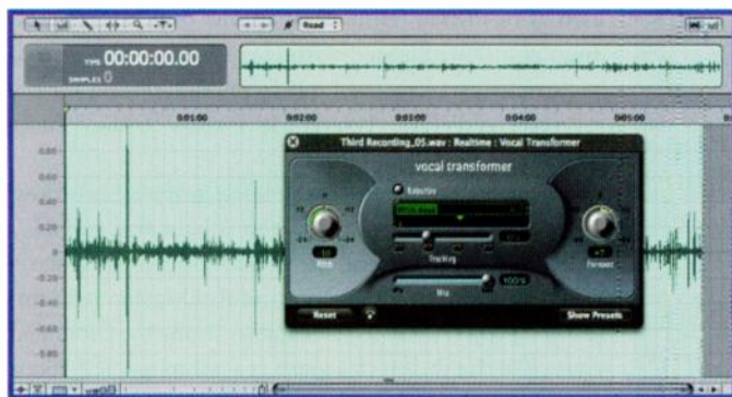
FIG. 1: Time- and pitch-manipulation effects such as Soundtrack Pro's Vocal Transformer usually offer independent control over pitch and formant.
