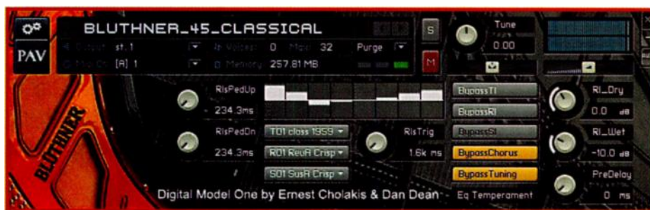
Blüthner Digital Model One's control panel is primarily devoted to choosing timbral, reverb, and sustain impulse-response presets.
