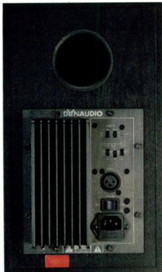
FIG. 2: The monitor accepts XLR connections only and has slider switches to control its highpass filter, level setting, and EQ adjustments.
