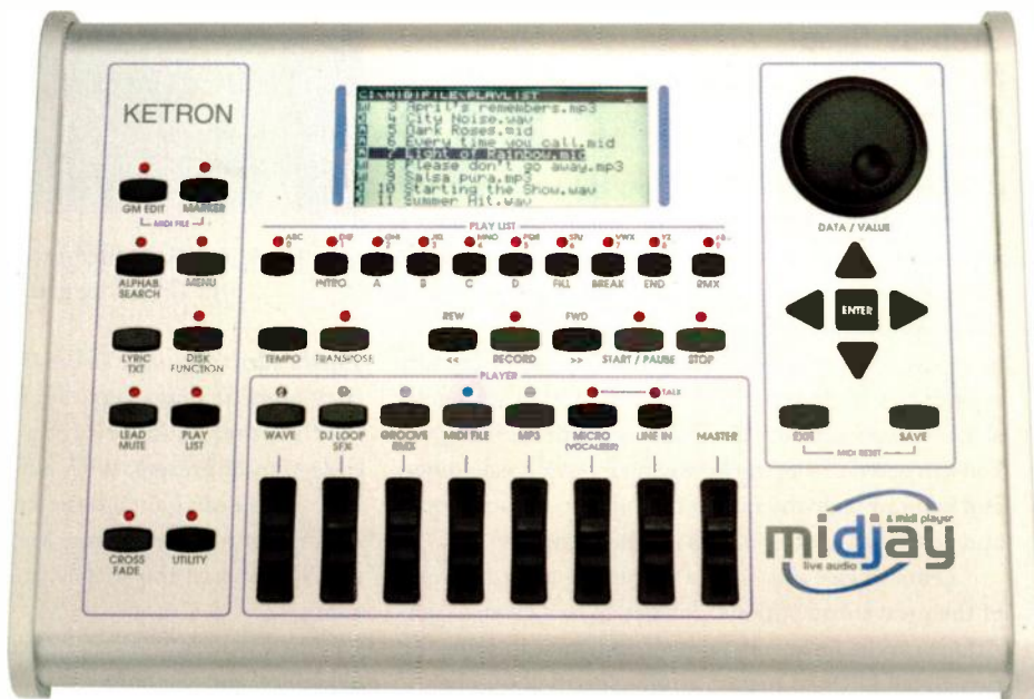
FIG. 1: The Midjay combines the functionality of a performance-oriented sequencer with a multitimbral sound module. Its faders control the volume level of MIDI and audio files, and the Master fader handles output on a global basis.
