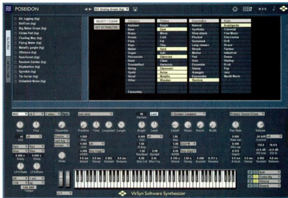
FIG. 1: Poseidon's main screen provides access to all the major program controls and displays a list of attributes for finding presets.
