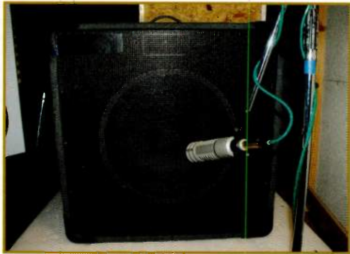
FIG. 3: In this photo, an Electro-Voice RE20 points between the center and the edge of the bass speaker. Note how it's angled slightly toward the middle to increase high-end definition and achieve a balanced sound.
