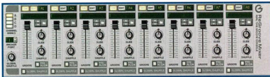
FIG. 3: The ReGroove Mixer lets you apply up to 32 different quantizing grooves to individual lanes.
