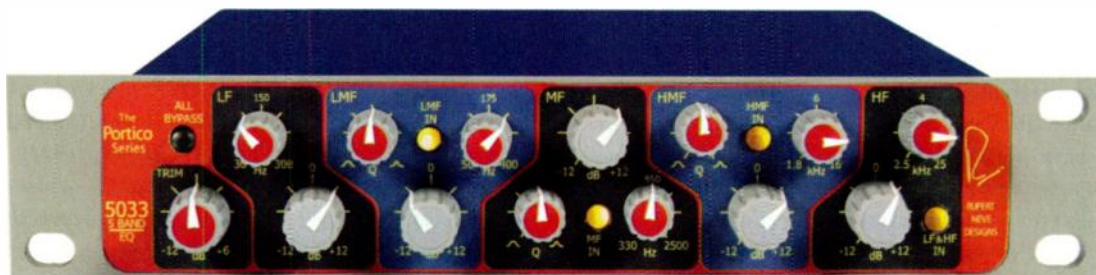
FIG. 1: The Portico 5033's front panel is replete with continuously variable rotary controls and backlit push-button switches.
