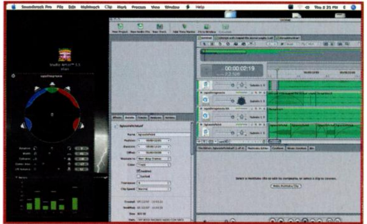
FIG. 2: The Surround Panner HUD offers parameters you can automate and is an efficient work area for surround mixing.
