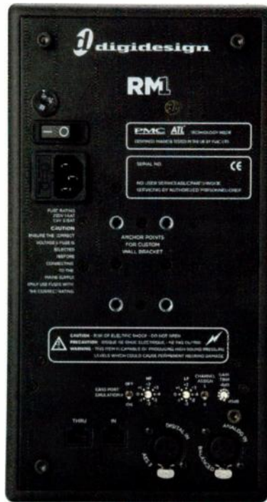
FIG. 2: The RM1's rear panel supplies XLR connectors for analog and AES3 digital input, along with RJ45 jacks for passing digital audio to or accepting it from another RM1.
