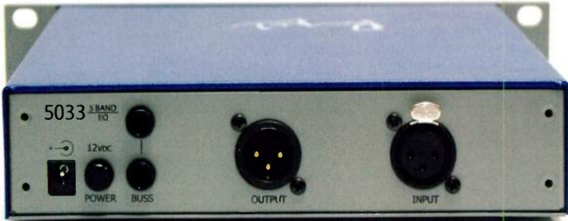
FIG. 2: Bus jacks on the 5033's rear panel facilitate interconnection with other units in the company's Portico line.
