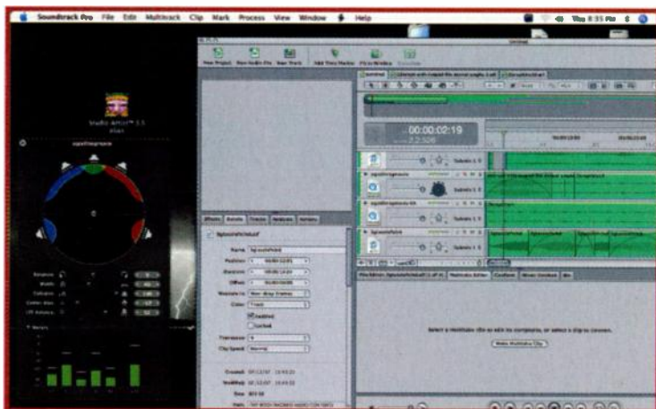
FIG. 2: The Surround Panner HUD offers parameters you can automate and is an efficient work area for surround mixing.
