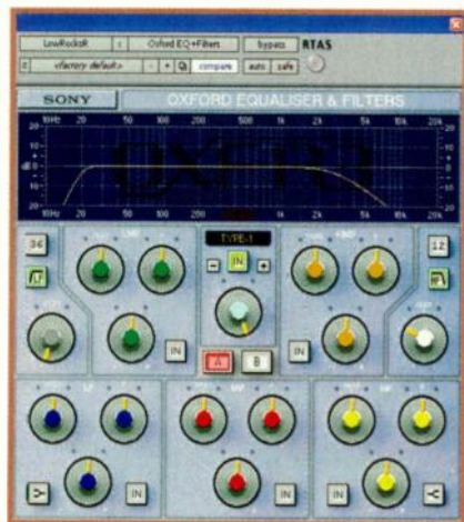
FIG. 2: A multiband equalizer’s lowest and highest bands often default to high- and lowpass filters, respectively.
