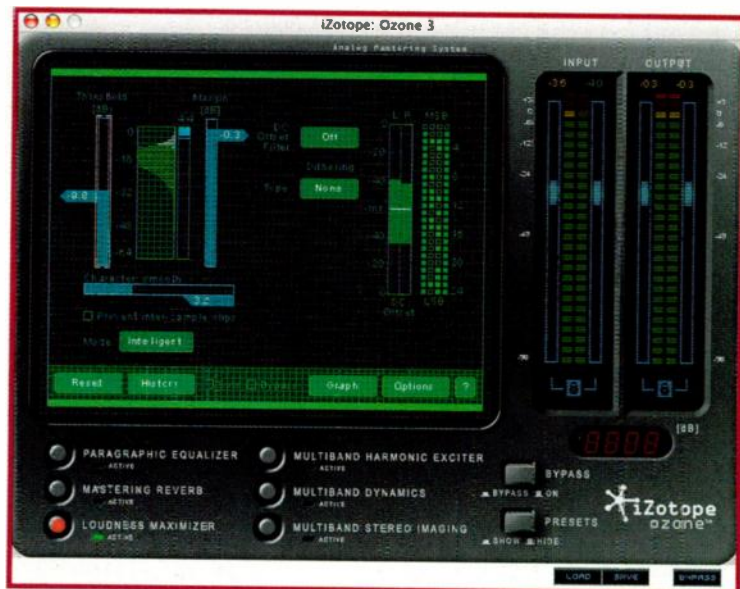
FIG. 3: This screen from iZotope Ozone shows six different metering functions: a histogram to the right of the threshold control, a gain-reduction meter, a DC offset meter, a bit scope, and input and output level meters with clip indicators.
