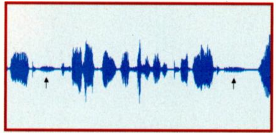
FIG. 2: The arrows point to the breaths in this waveform display from an interview track.
