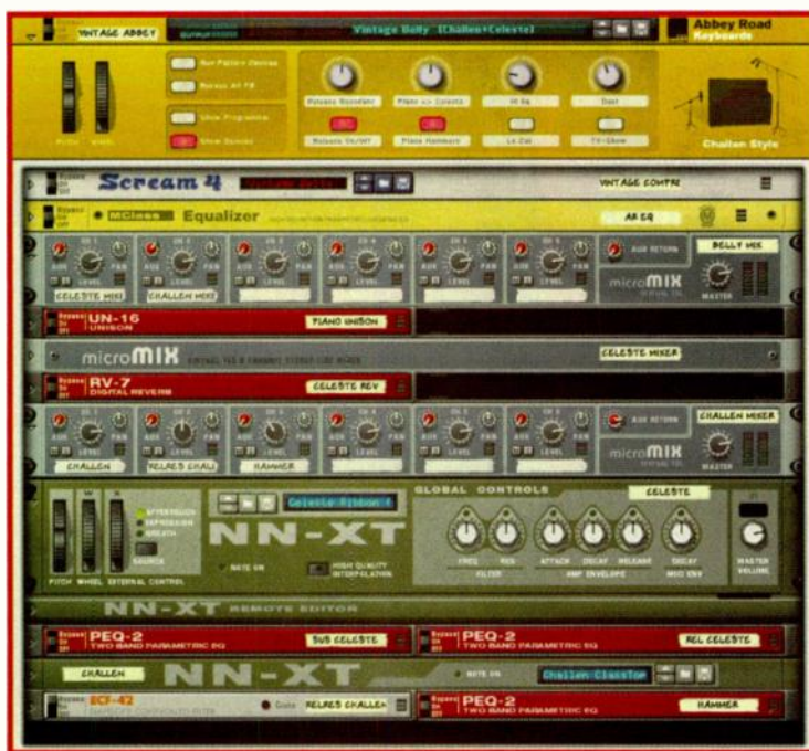
Abbey Road Keyboards' Combinator patches combine multisampled NN-Xt patches for individual mic placements with mixing, effects processing, and global controls.
