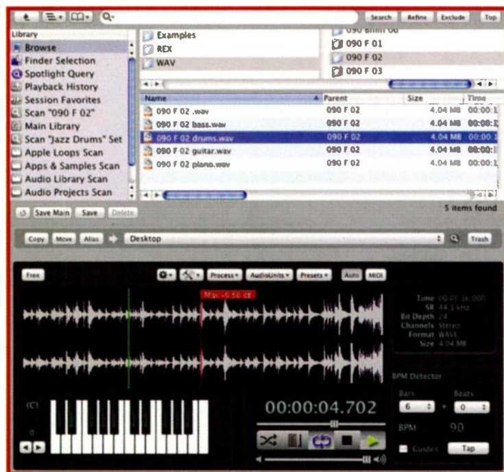
AudioFinder's one-window GUI includes a Library panel, a dual-format browser, and an audio-file viewer and player.
