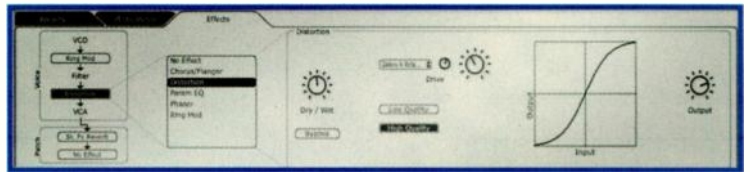
FIG. 3: The effects section includes both voice effects, which are inserted into the synthesis chain, and patch effects, which occur at the instrument's outputs.
