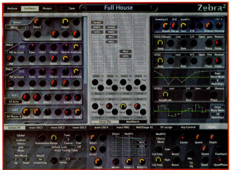
FIG. 1: The signal-flow grid in the center of Zebra's Synthesis tab is flanked by a sound-module rack (left) and a modulator-module rack (right). The Global/FX tab in the bottom panel reveals Zebra's modular effects processor.
