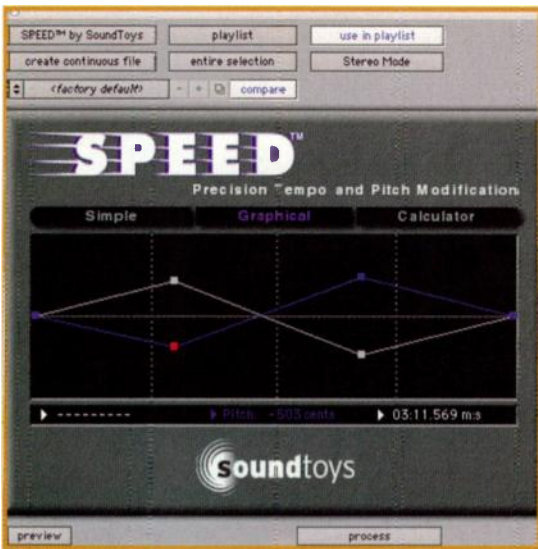
FIG. 3: Speed allows you to change the pitch and tempo of a sound independently.
