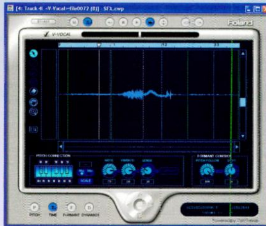
FIG. 2: Sonar's V-Vocal offers a graphical environment for altering pitch, timing, volume, and formant.
