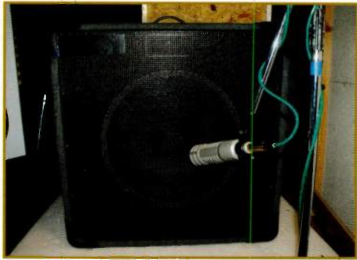
FIG. 3: In this photo, an Electro-Voice RE20 points between the center and the edge of the bass speaker. Note how it's angled slightly toward the middle to increase high-end definition and achieve a balanced sound.
