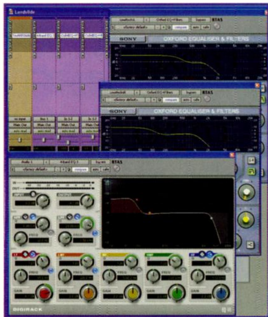
FIG. 6: Sometimes a heavy hand is warranted, as with these three EQ plug-ins adding up to 10 dB of low bass to the primary rumble tracks.
