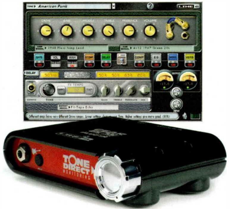
FIG. 1: The Gold and Silver bundles both come with a combination dongle and instrument interface called the TonePort DI.
