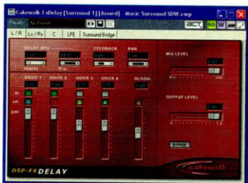
FIG. 1: Sonar's SurroundBridge makes any mono or stereo plug-in available as a selectively linked set of processors on a surround bus.
