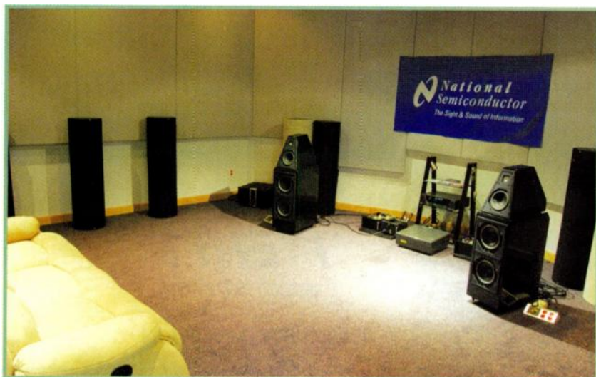
FIG. 1: National Semiconductor's sound room is completely isolated and acoustically treated. The finest consumer speakers are used to evaluate the performance of devices built with the company's audio chips.
