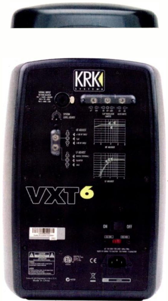
FIG. 2: The switches for EQ, clip indication, and automute are protected by covers so that they can't be accidentally changed.
