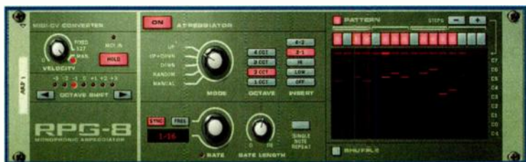
FIG. 1: The RPG-8 arpeggiator features a rhythm-pattern sequencer, octave shifting and repeating, several Insert modes, and the option to not repeat single notes.
