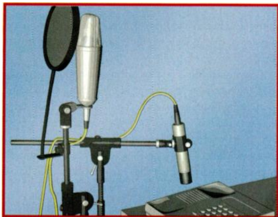
FIG. 1: This drawing shows the basic setup for the miking-the-speakerphone method of phone-interview recording.
