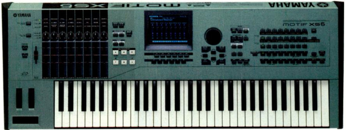
FIG. 1: The Motif XS's front panel just screams "user control." The eight sliders let you control the volume of various sound elements. The knobs have multiple assignments, and the buttons on the right choose tracks, Voices, or other objects, depending on the current mode.
