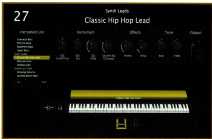
FIG. 4: MainStage gives you a performance rig for Logic Pro and AU plug-ins without the encumbrance of running Logic.
