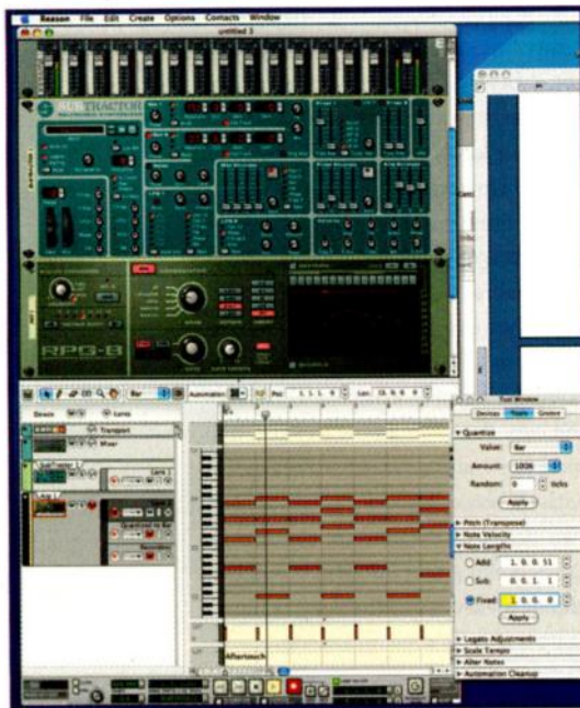
FIG. 4: The Note Lengths tool is useful for maintaining precise durations for RPG-8 chord-progression sequences.
