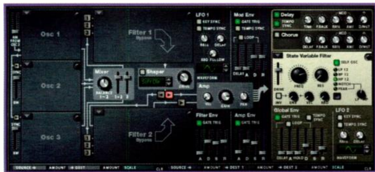
FIG. 1: Oscillators, filters, and polyphony are disabled when using Thor exclusively as a filter device.
