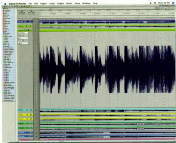
FIG. 4: A brickwall limiter adds distortion to a track when it squares off the top of its waveform on peaks.
