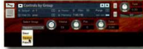
➤ FIG. 3: Use a menu to have the same GUI elements control different groups.
