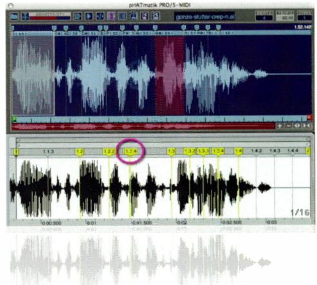
➤ FIG. 1: This composite screen shot shows two approaches to aligning syllables to the beat: slicing in iZotope Phatmatik Pro and using Warp markers in Ableton Live.
