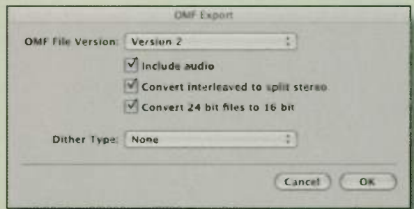
Step 4: When exporting an OMF, convert all files to a common bit depth to ensure compatibility.
