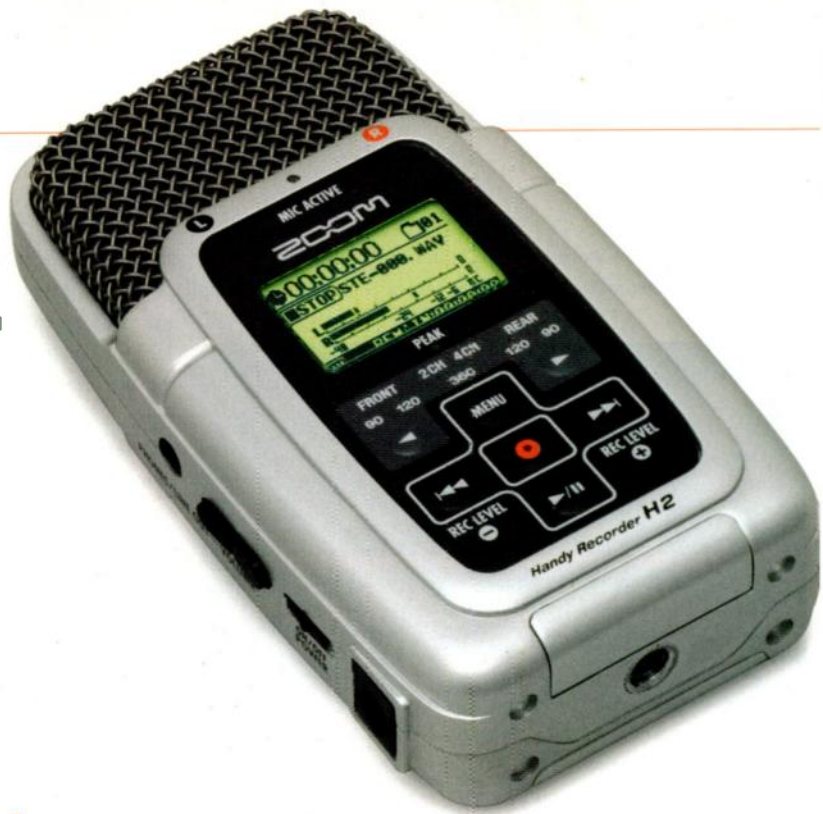
FIG. 1: The pocket-size Zoom H2 has four onboard microphones and records 2- or 4-channel audio at rates as high as 96 kHz. Most controls and the backlit graphic display are on the front panel.
