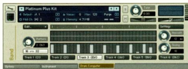
FIG. 3: In Play mode, each of Kontakt's drum kits includes a 6-sound, 32-step drum sequencer with a graphical interface for editing Velocity and pitch.
