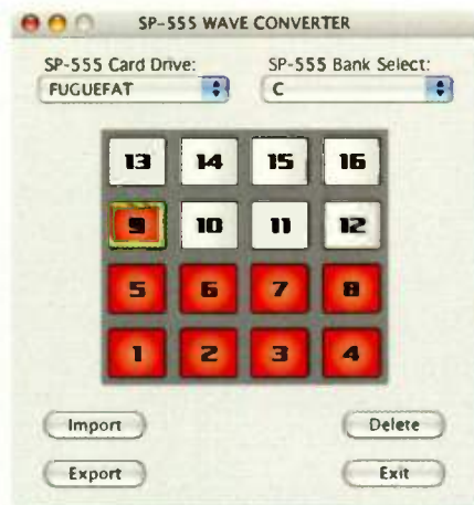
»» FIG. 3: The rudimentary Wave Converter lets you transfer samples between the SP-555 and a Mac or PC. You need a CompactFlash reader to use it, though.
