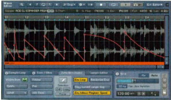
FIG. 4: Every sample in Kontakt can have its own Zone Envelopes, which can be edited in this graphical interface. Note the segment curvature and the easy snapping of the envelope points to sample slice points.
