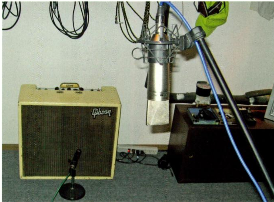
FIG. 2: If you place the mics properly, you can create an effective stereo mix of a mono electric guitar.
