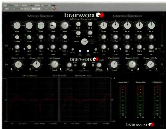
Brainworx bx_digital is a software simulation of the company's hardware mastering processors. The display includes a large, well-marked depiction of the EQ curve for each channel.
