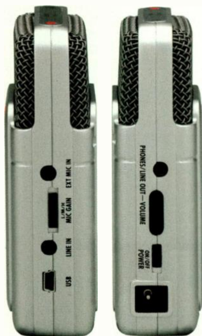
FIG. 2: The H2's side panels provide a stereo mic input, stereo line input, and stereo headphone output, all on 3.5 mm jacks, as well as connections for the included AC power adapter and USB 2.0.
