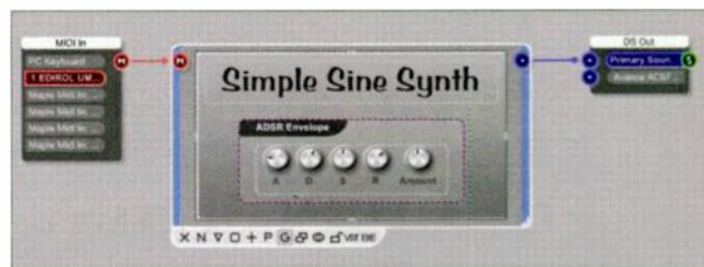
FIG. 3: The simple sine-wave synth of Fig. 1 has been turned into a single Module with a functional panel. Clicking on VST or EXE on the tab beneath the Module will turn this Module into a VST plug-in or a standalone Windows application.
