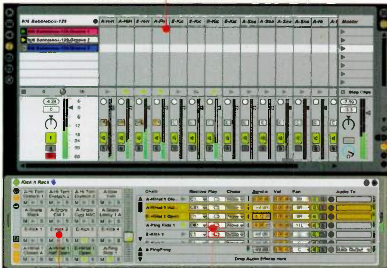
➤➤ FIG. 1: Drum Racks map plug-in instruments to individual pads triggered by MIDI notes. Racks have their own send effects and submixer.
