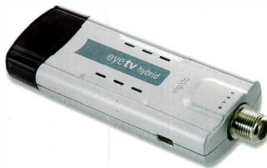
FIG. 1: Elgato's EyeTV Hybrid plugs into a USB 2.0 port on a Mac and has connections for composite and S-Video cables from external video sources, as well as a coax connector to handle cable TV channels.
