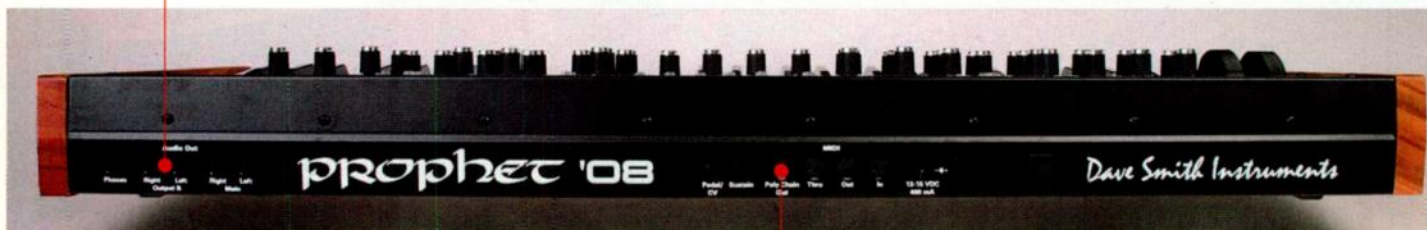
➤ FIG. 2: In addition to the expected main outputs, pedal jacks, and MIDI ports, the Prophet '08's sparse rear panel furnishes a pair of separate outputs for the second layer of sounds.
