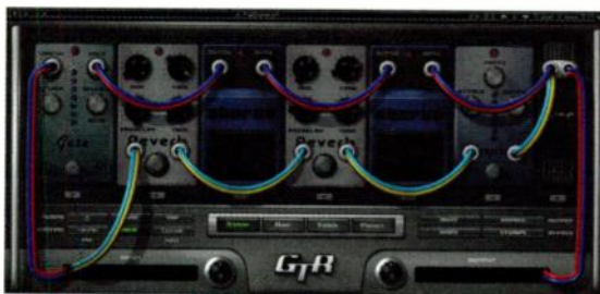
FIG. 3: With View mode selected in Tool Rack's Stomp tab, you can see the current cable routing and select from three different routings for the effects, both before and after the amplifier.
