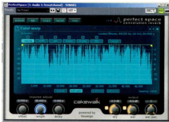
FIG. 3: Unlike some other programs, Sonar's Perfect Space imposes no limits on the length of the IR. The IR shown here lasts 45 seconds.
