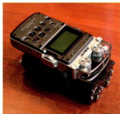
FIG. 3: This is the PCM-D50 mounted on Sony's optional XLR-1 adapter.
