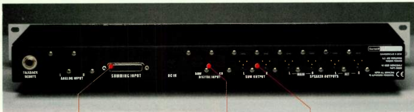
» FIG. 2: Most of the D-Box's I/O is on XLR jacks, with the exception of the eight summing inputs, which are on a DB-25 connector.
