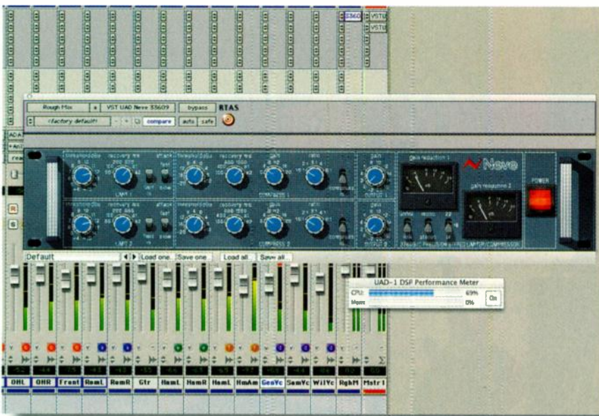
FIG. 2: UAD Meter shows how much of the Xpander's processing power and RAM is being used.
