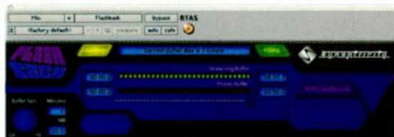
Flashback is an RTAS and AudioSuite plug-in that records everything you do into RAM for up to 15 minutes at a time.
