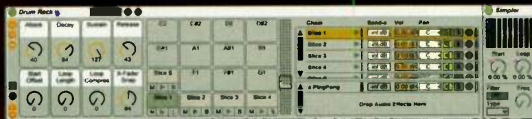
FIG. 1: In a Drum Rack, each pad corresponds to a MIDI note. Sixteen pads are visible at a time, and supported MIDI pad controllers always play the visible pads.
