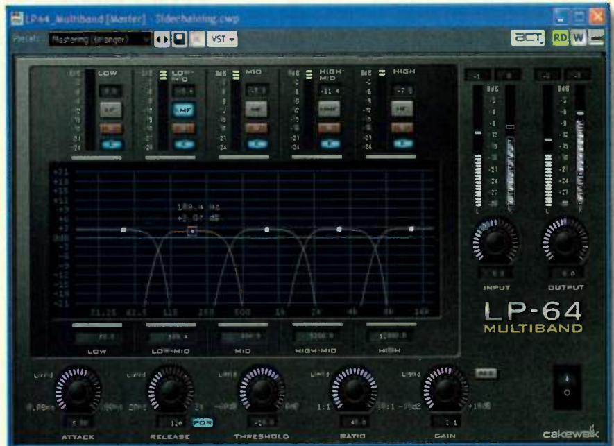
FIG. 3: The LP-64 Multiband compressor offers transparent linear-phase multiband compression suitable for bus compression or mastering.
