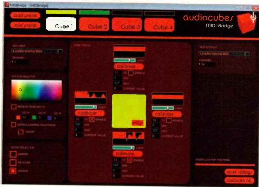
FIG. 3: MIDI Bridge translates sensor data from the AudioCubes to MIDI Control Changes or notes. It also converts MIDI data from a computer-based sequencer to color values for the cubes' internal LEDs.
