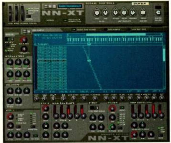
FIG. 1: When a REX file is loaded into the Reason NN-XT sampler, each slice will be assigned to a separate key. Use the Out knob (middle right of graphic) to assign slices to various audio outputs, such as the 5-6 stereo pair (shown here).
