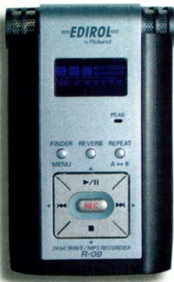
FIG. 1: Edirol's R-09 is small enough to operate with one hand, yet it offers pro-level features such as a digital audio out and support for SD cards up to 16 GB.
