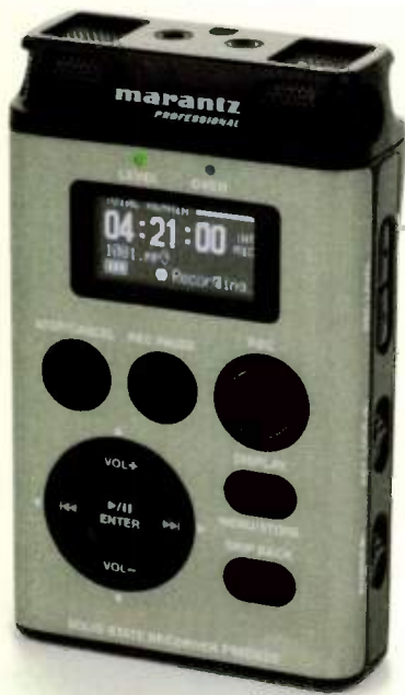
➤➤ FIG. 3: The latest in a long line of portable recorders from Marantz, the PMD620 is quick on the draw and offers the ability to save and name user presets containing setup parameters.
