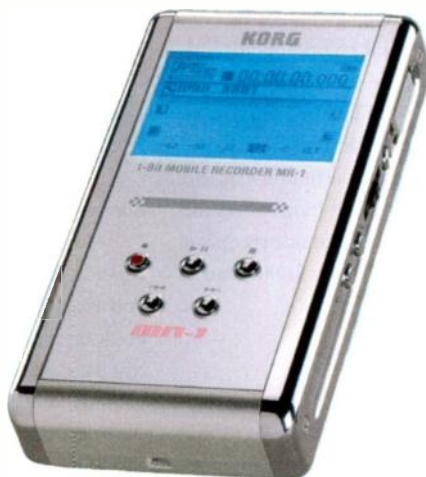
FIG. 2: The Korg MR-1 delivers the highest-quality audio performance of all the recorders in this roundup, and it's the only one with an internal hard disk.
