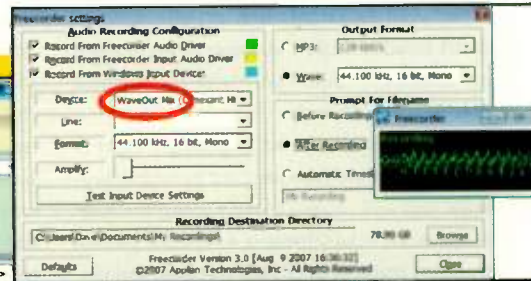
Step 3: To capture the vocal stylings of Web sites or nonrendering software, resample the PC's WaveOut Mix (t.nyurl.com/2u3t4j).
