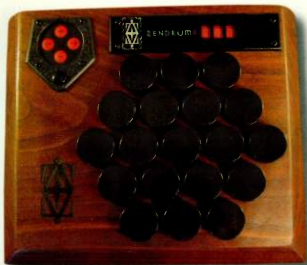
»» FIG. 1: The ZAP's spartan interface includes 19 hard plastic triggers neatly arranged in five rows.
