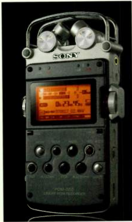
▶▶ FIG. 6: Although slightly larger than its competitors, the Sony PCM-D50 offers all the features you'd want in a portable recorder, including 4 GB of onboard memory and 12 hours of 96 kHz record time on a single set of batteries.
