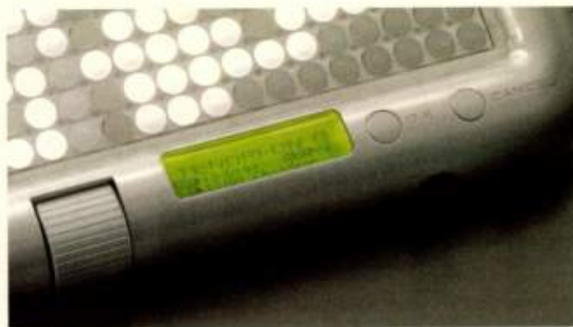
FIG. 2: You control transport functions and access menus in the Tenori-on's LCD using just two buttons and a jog wheel.
