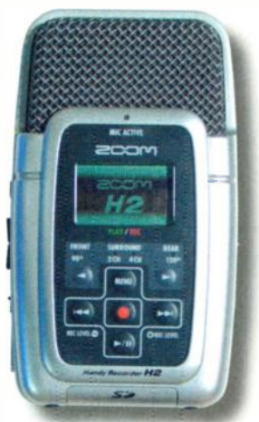
FIG. 8: With four built-in mic capsules, a metronome, and a versatile tuner, the Zoom H2's 360-degree recording and low cost make it unique among its competitors.
