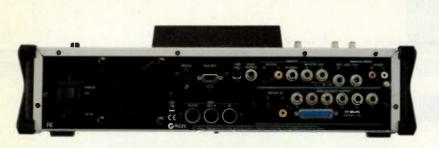
FIG. 2: The MV-8800's back panel offers analog audio I/O, S/PDIF out, MIDI and USB ports, and connections for a monitor, mouse, and footswitch. Also shown here is the optional MV8-OP1 expansion.
