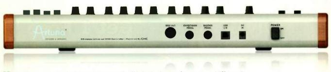
≫ FIG. 3: You can choose an optional 12V DC adapter to power the AFE keyboard, or draw power from your computer's USB connection.
