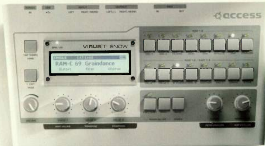
»» FIG. 1: The Virus TI Snow's compact configuration of knobs and buttons provides quick access to programs and their essential parameters.
