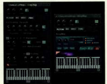
FIG. 6: FL Studio's BeepMap will convert an image to any number of partials you specify. All of its controls operate in real time.
