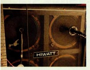
FIG. 3: Here, a pair of mics are aimed at the middle of the speakers of a guitar cabinet.
