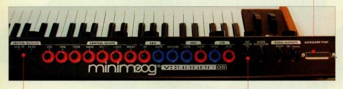
**>>** Keyboard gate and CV outputs allow you to interface with external instruments.
