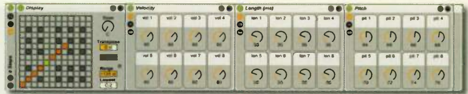
➤➤ FIG. 1: In this 8-step sequencer, the Scale effect at the left displays the active step in green, and the Macro controls of the three MIDI Effect Racks control the step Velocities, lengths, and pitches.
