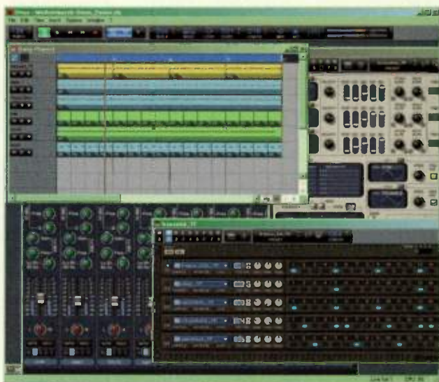
»» FIG. 1: Orion provides more than a dozen sound generators, lots of effects, and capabilities for sequencing, audio recording, and mixing.
