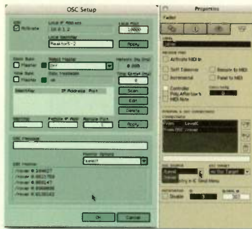
FIG. 3: Reaktor's OSC Setup panel (left) shows OSC coordinates and displays incoming messages. The Properties panel (right) is where you create an OSC hook, which binds the fader's position to values received from the rover curve in IanniX.
