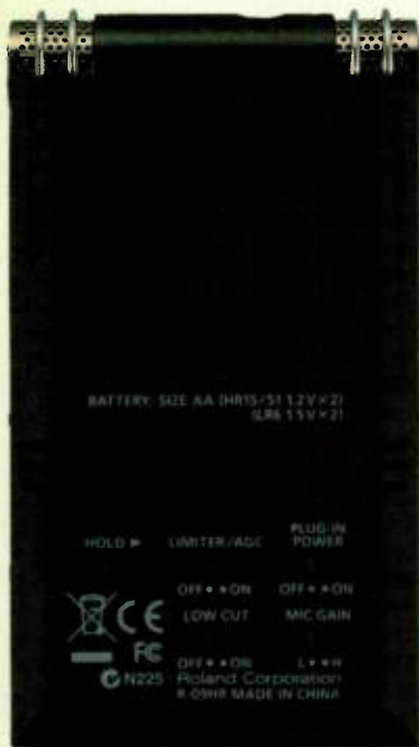
» FIG. 2: On its rear panel, the R-09HR provides a built-in speaker, a mic sensitivity switch, a battery compartment, and controls that activate a low-cut filter, 5V plug-in power, a hold function, and a user-selectable limiter or AGC.
