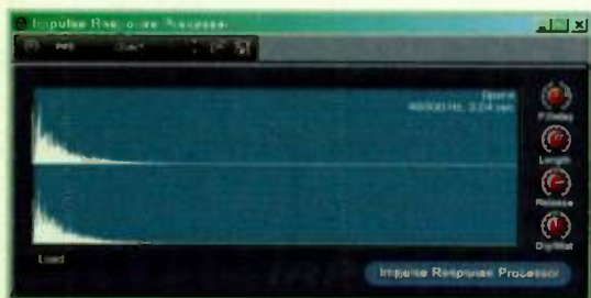
» FIG. 2: Orion's convolution reverb is a relatively new addition to the program. Several other reverbs are available if you're short on CPU and don't need the convolution capabilities.
