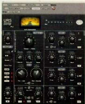
Input and output controls on the left, compression in the center, and EQ on the right give you many channel strip options in Classic Console Strip Pro.
