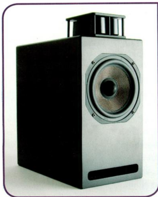
FIG. 1: The S7 includes two LET tweeters facing front and back and one 6.5-inch midrange that can reproduce frequencies down to 45 Hz. The crossover frequency is about 3 kHz, and the input impedance is flat ( \pm 1\Omega ) across all frequencies. Notice how the LET diaphragm on top of the speaker is actually two hemicylindrical membranes.
