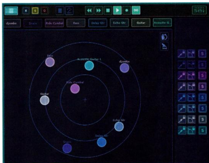
FIG. 2: You adjust the positions of eight channels at a time on the Surround page.
