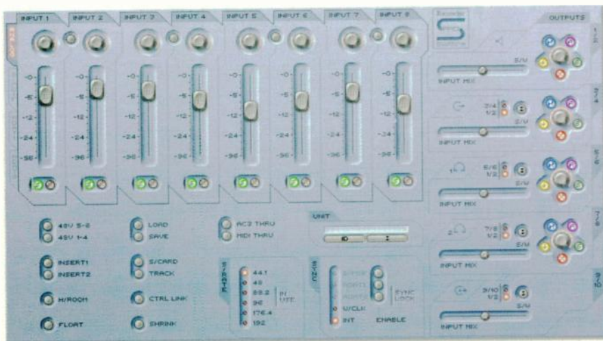
FIG. 1: The SaffireControl Pro software provides onscreen control of the digital mixer and many other features.
