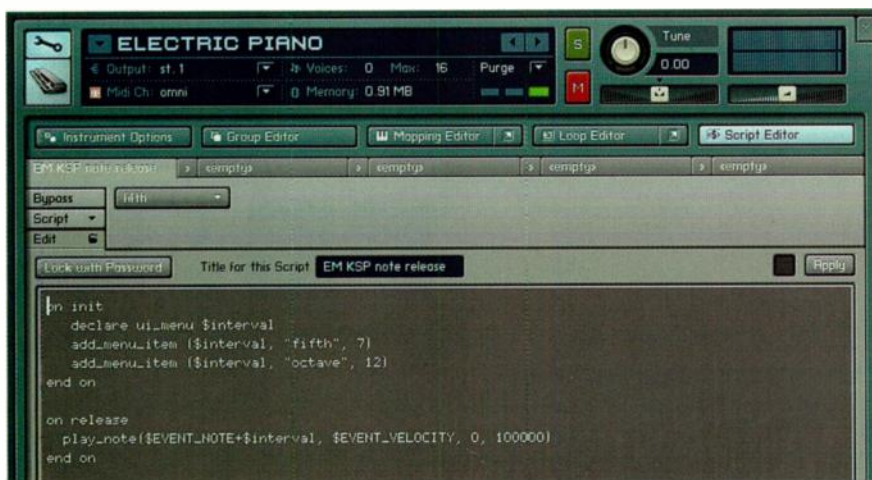
FIG. 2: This figure shows a Kontakt script that will add a second note—either a fifth or an octave—above the note that is played. Up to four additional scripts can be added to the slots that are marked "<empty>."
