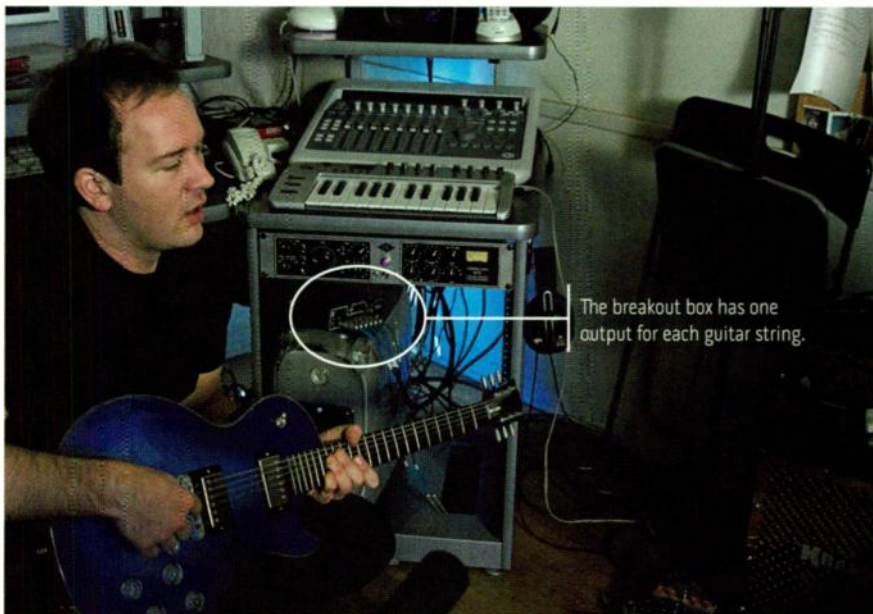
FIG. 2: Small in his personal studio demonstrating how the Gibson HD.6X-Pro Digital Les Paul utilizes the breakout box with the six outputs. Also visible is the Universal Audio 6176, the M-Audio 02, and the DigiDesign Digi 003.
