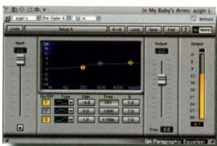
FIG. 3a: The Waves Q10 EQ plug-in is used to apply a shelving cut to low frequencies on an acoustic guitar track in order to make room for bass and kick in the mix.
