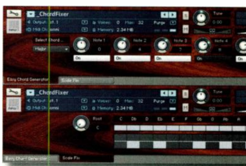
FIG. 4: In this 2-script instrument, the first script (top panel) turns notes into chords, and the second script (bottom panel) keeps those chords within a user-defined scale or mode.
