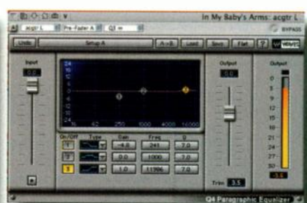
FIG. 3b: The low-shelving band is bypassed on the acoustic guitar track, restoring its bass frequencies, when drums and bass temporarily drop out of the mix.
