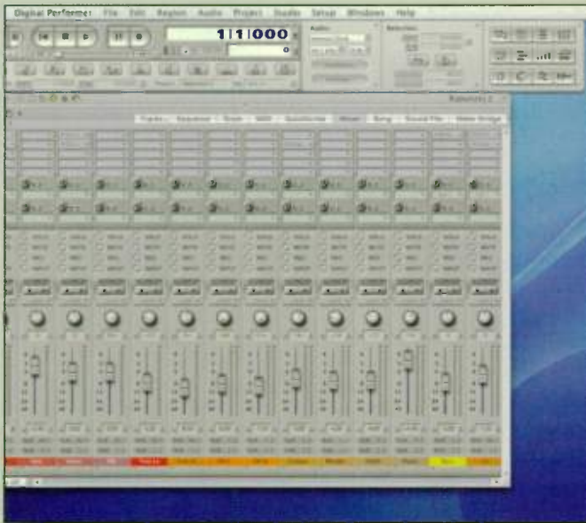
Step 3: Take a screen shot of your mixer to remember panning, levels, and sends.
