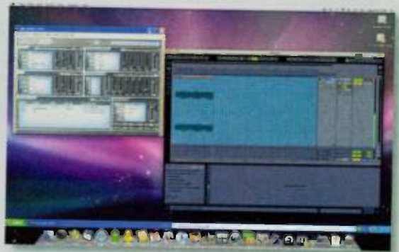
FIG. C: When running in Parallels Coherence mode, your Windows applications open directly inside OS X.
