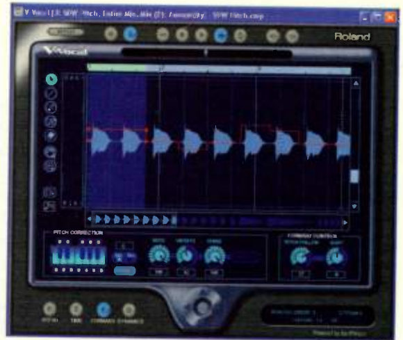
FIG. 1: Cakewalk Sonar's V-Vocal Pitch Follow control determines how the formant tracks pitch changes. The formant envelope lets you fine-tune the results.
