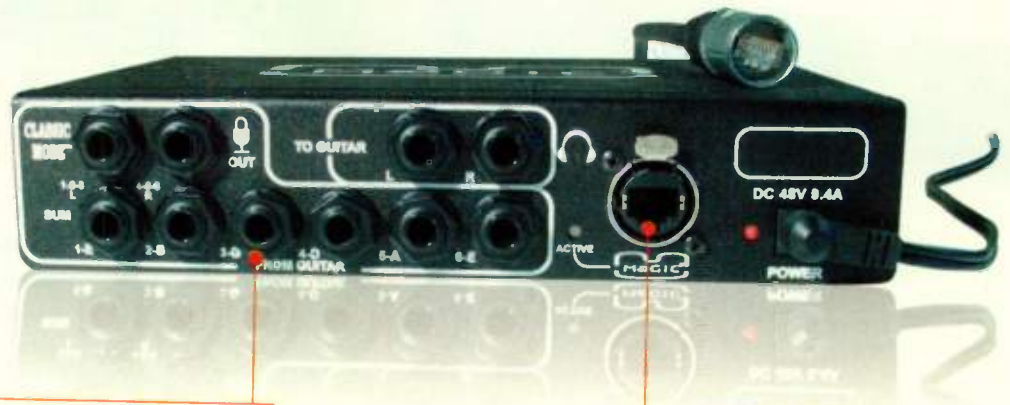
➤➤ FIG. 2: The BoB breakout box outputs signals from the HD.6-X Pro's six strings in mono, stereo, and Hex modes. It can also route a cue feed to and accept a mic signal from the guitar's jack plate.
