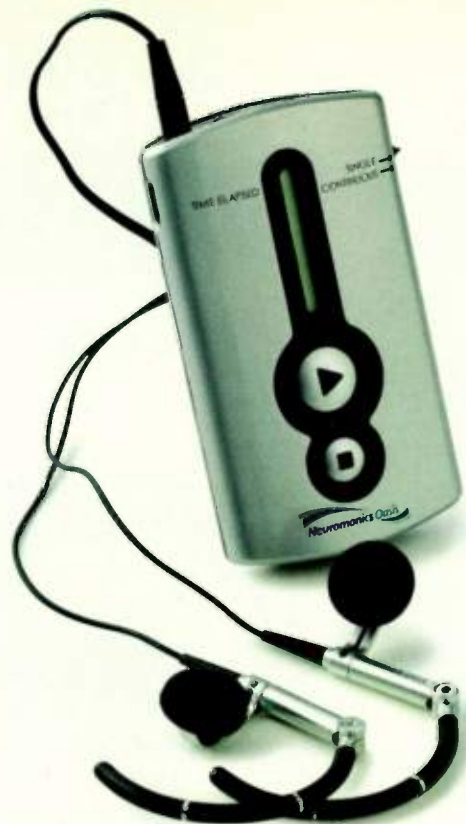
FIG. 1: The Neuromonics tinnitus treatment relies on a small, portable device that plays customized noise and music to mask the symptoms of tinnitus. The audio signal is programmed by an audiologist or physician according to the patient's hearing profile.
