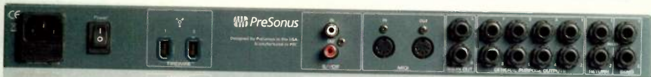
FIG. 2: The FireStudio Project's rear panel includes eight General Purpose analog outputs you can use to create mono or stereo mic headphone mixes.
