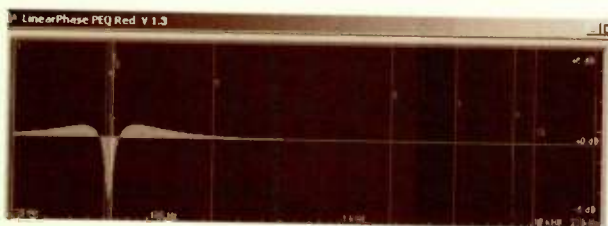
FIG. 3: This example shows how Katz dipped a single offending bass note and added a slight shelf to enhance the level of a weak bass instrument.
