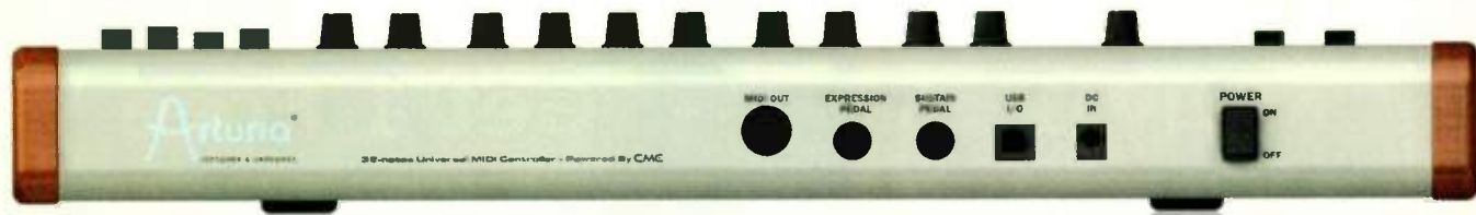
FIG. 3: You can choose an optional 12V DC adapter to power the AFE keyboard, or draw power from your computer's USB connection.
