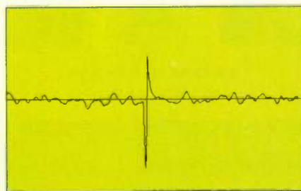
FIG. 2: A click is immediately apparent by its contrast with the surrounding music waveform, and intuitively just as easy to fix by interpolation.
