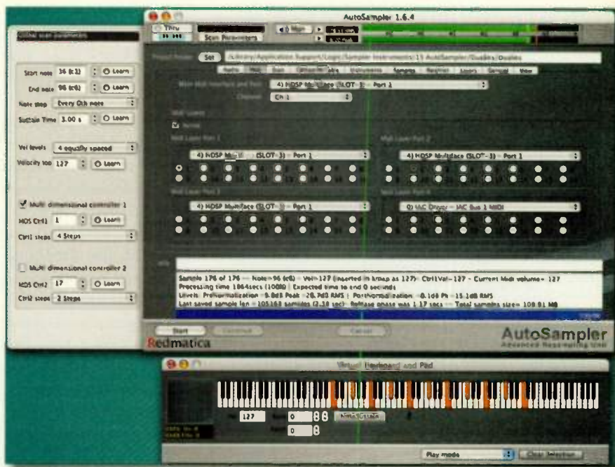
FIG. 2: You set the note and Velocity intervals along with MIDI layering conditions that AutoSampler uses to create a multisampled instrument.
