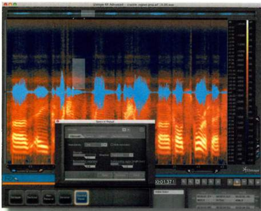
FIG. 5: iZotope RX's main view offers overlaid waveform and spectral editing views. RX's Spectral Repair module uses interpolation technology to fix audio glitches.
