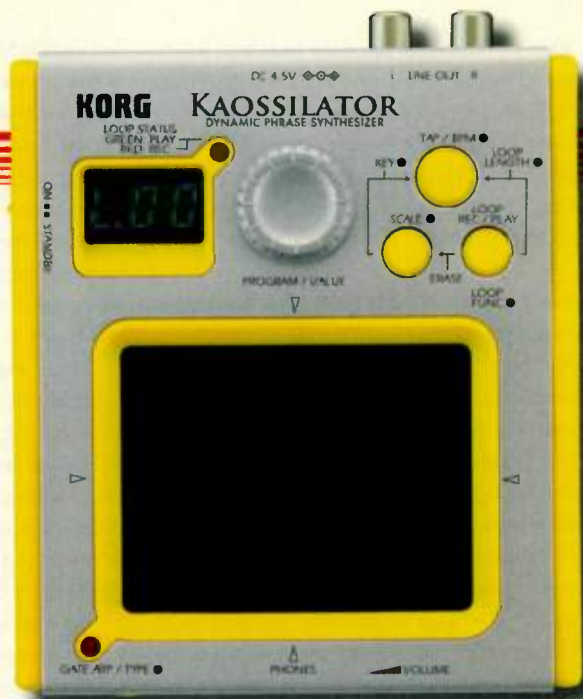
»» FIG. 1: With rich sounds derived from the Korg Radias, the battery-powered Kaossilator is a one-finger party to go. Its onboard audio looper lets you build 4-bar grooves through endless overdubs.
