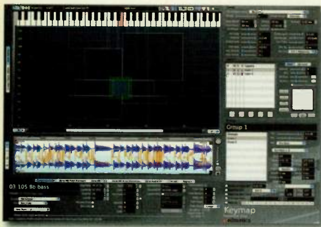
FIG. 3: Zones in each Keymap layer are automatically tiled as they are created. You can set up zone crossfades individually, as shown for the center zone here.
