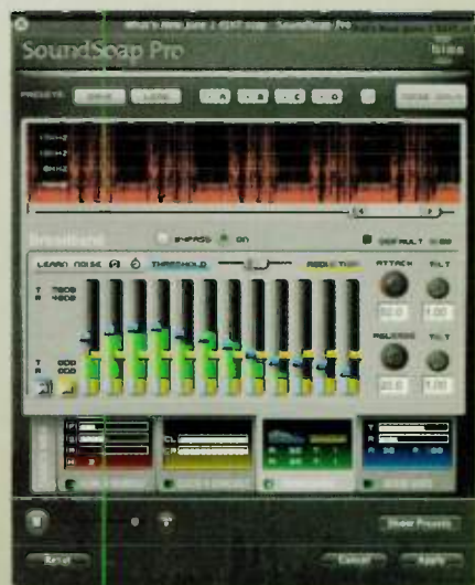
FIG. 1: BIAS SoundSoap Pro’s denoiser module offers both a “learn noise” option and another that extracts a profile from a user-specified section of the audio that includes both source and noise.
