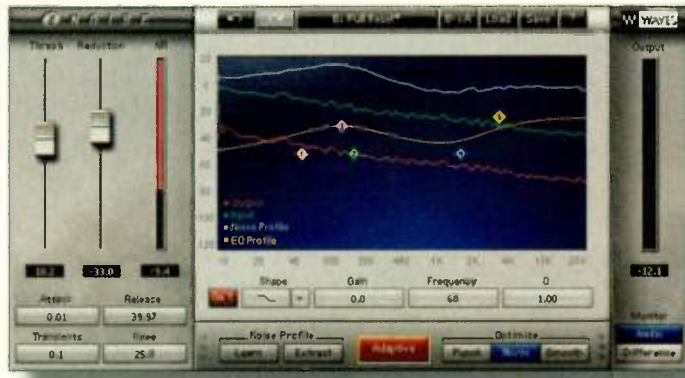
FIG. 3: Waves designed three presets into Z-Noise that let you tailor the plug-in's response depending on the transient character of the source audio.
