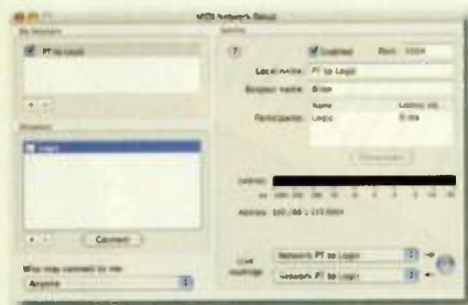
FIG. 2: This screen shot shows the configuration of a network MIDI port on a Mac. Since OS X 10.4, support for MIDI over LAN has been standard.
