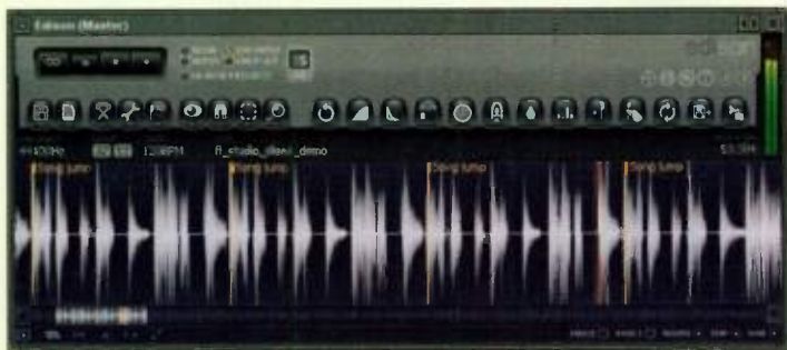
FIG. 2: The Edison audio editor is packaged as an effects plug-in, which lets you record and process audio anywhere you can place an effect.
