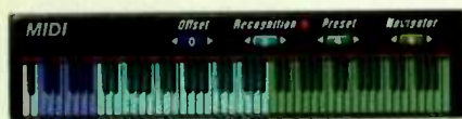
➤➤ FIG. 2: The MIDI keyboard panel replaces the area below the faders and lets you issue commands or enter notes and chords.
