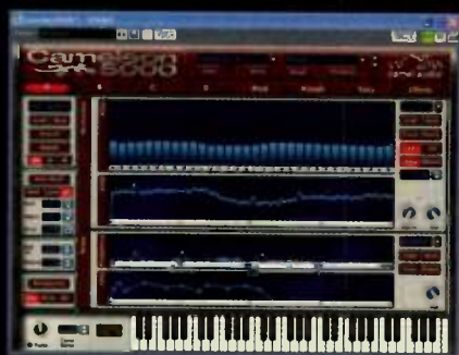
FIG. 2: Cameleon displays the converted image using adjustable sliders that represent the amplitude for each partial (top). A separate set of sliders is available for adjusting the noise components (bottom).
