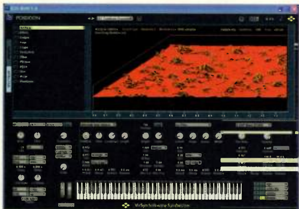
FIG. 8: Poseidon lets you choose how you want to display the spectrum of the image you import. The 3-D waterfall view is shown here.
