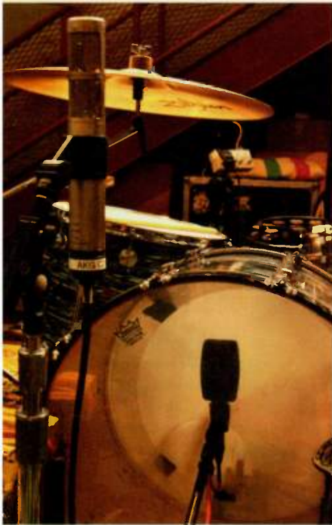
FIG. 1: Steve Albini uses a stereo mic in front of the kit and often mics both sides of the kick and toms.
