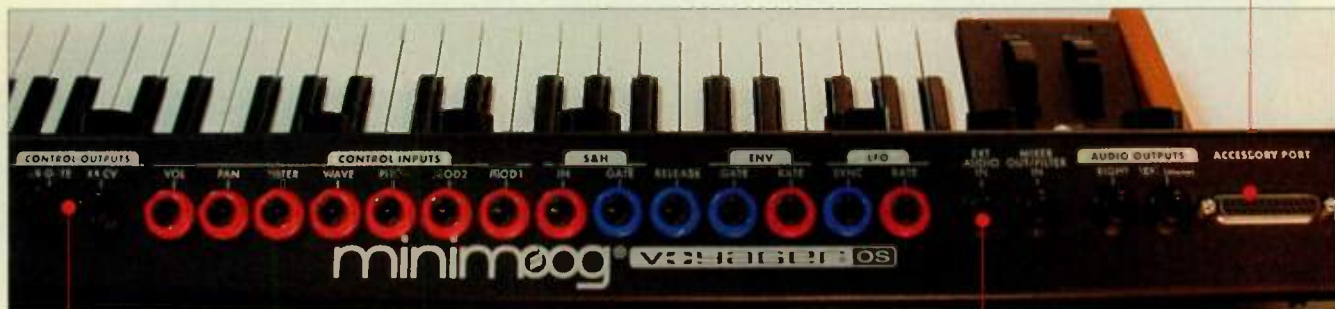
FIG. 2: The Voyager OS's jack panel offers impressive analog connectivity for control-voltage and audio signals.
