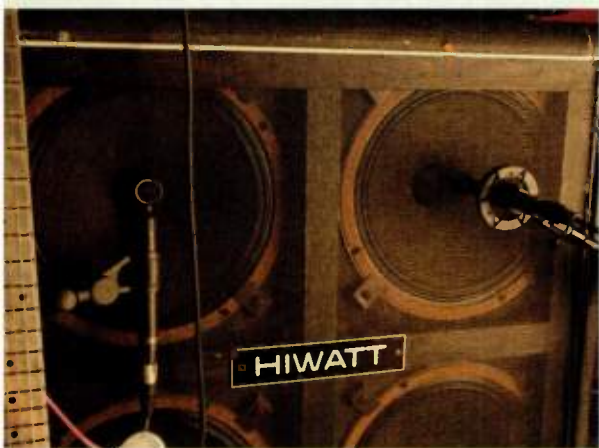
FIG. 3: Here, a pair of mics are aimed at the middle of the speakers of a guitar cabinet.
