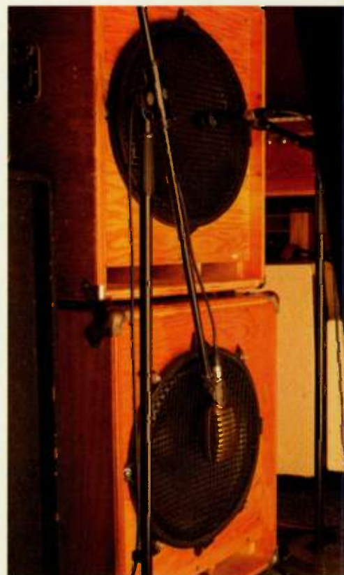
FIG. 2: Albini combines two different mics on a bass rig in order to capture a wide frequency spectrum.
