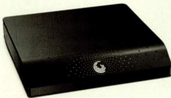
External SATA (eSATA) drives can provide better speed than either USB 2.0 or FireWire hard drives. The Seagate FreeAgent Xtreme (above) includes all three types of connectors on the rear panel (right).
