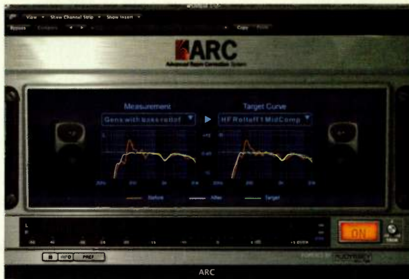
»» FIG. 1: The ARC plug-in EQ's your playback system to give it a flat response based on the curve generated by the measurement application and the optional Target Curve.
