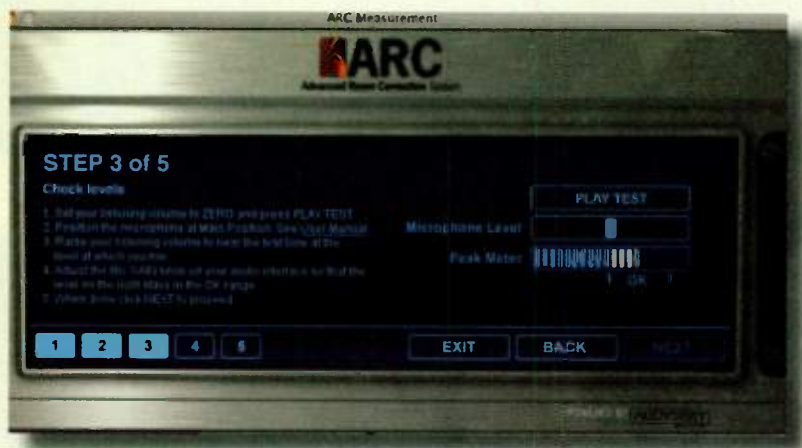
FIG. 2: The room measurement application features step-by-step onscreen instructions that guide you painlessly through the process of measuring your room's acoustics.
