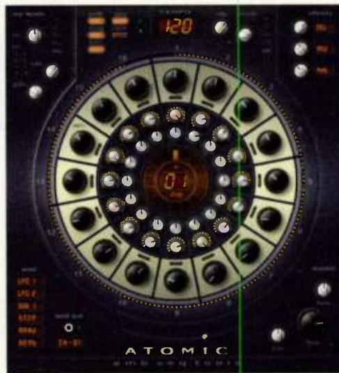
FIG. 1: Atomic combines a 16-step sequencer, an arpeggiator, an analog-modeled synth, and three effects.
