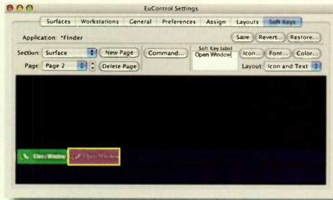
FIG. 3: The included EuControl software's soft-key editor allows you to create assignable buttons that appear on the MC Control's touch screen.
