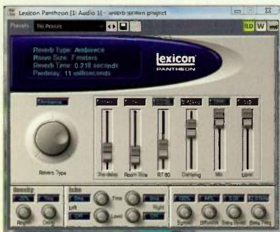
FIG. 3: Using a reverb with a decay time of less than 1 second—such as this setting on Lexicon's Pantheon plug-in—helps keep reverb wash from cluttering up a mix.
