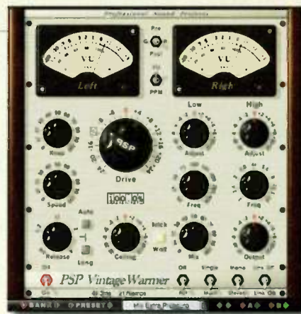
FIG. 3: VintageWarmer 2's controls are designed to emulate warm, analog-tape-style compression.
