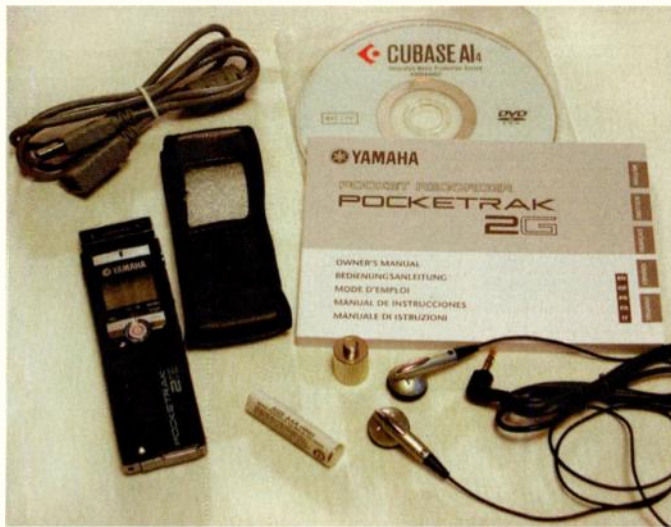
FIG. 2: Included with the Pocketrak 2G are a leather carrying case, a USB extension cable, a rechargeable AAA battery, earbuds, a stand adapter, a manual, and Cubase AI 4 software.
