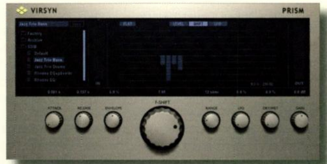
FIG. 1: This acoustic bass setup shifts bands 750 through 1,100 Hz down by varying amounts within a 7-semitone range.
