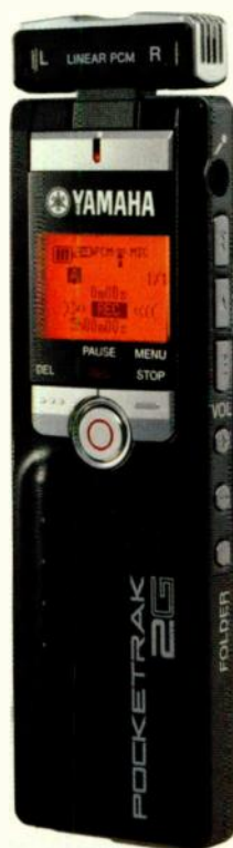
FIG. 1: The Pocketrak 2G offers advanced features such as an adjustable mic, a built-in speaker, and a slide-out USB connector—all within an ultraslim, lightweight profile.
