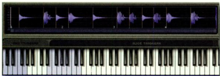
FIG. 2: The first 16 notes of Beatscape's keyboard, starting at C3 (Note Number 36), trigger the 16 pads. Each pad's audio slices are mapped to MIDI notes starting at E4 (Note Number 52) on the channel corresponding to the pad's number.
