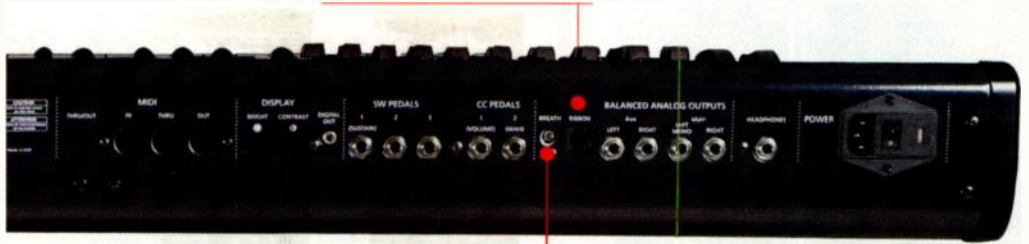
FIG. 2: In addition to its audio, MIDI, and sync ports, the PC3x has plenty of controller inputs, including ports for three switch pedals, two continuous controller pedals, a breath controller, and Kurzweil's optional Super Ribbon Controller.
