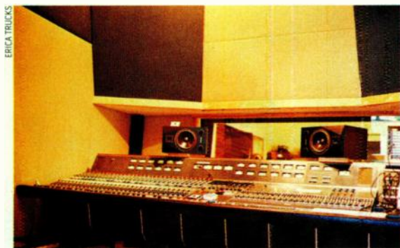
FIG. 2: Trucks's control room features a vintage Neve 8048 console, which was formerly used at Ray Davies's Konk Studios in London.
