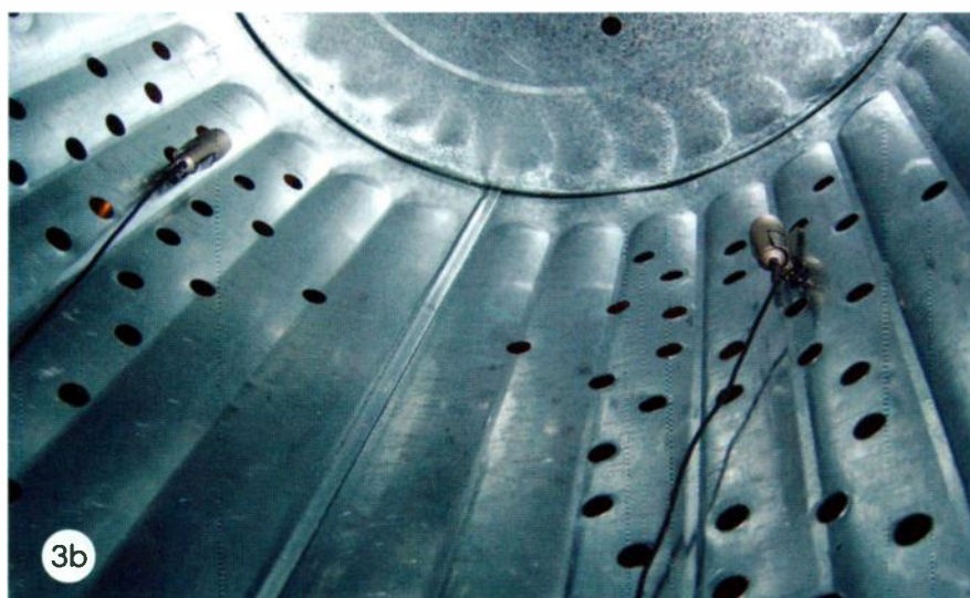
FIGS. 3a and 3b: I used a trash can as a filter on a piano (3a). Notice how the mics are pointed away from the source to catch reflections off the bottom of the can (3b).
