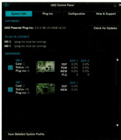
FIG. 2: UAD Control Panel helps you configure the plug-ins and monitor the performance of the DSP cards.
