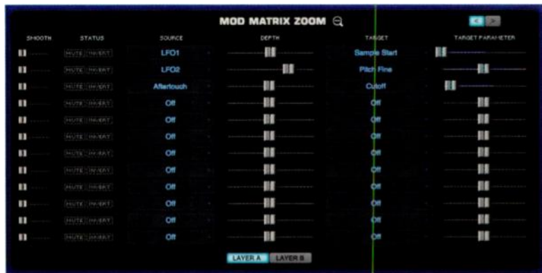
FIG. 3: Omnisphere organizes all of the modulation routings for both Layers on the Mod Matrix Zoom page. The Smooth slider lets you slow a modulation source's output; experienced synthesists may recognize this function as lag.
