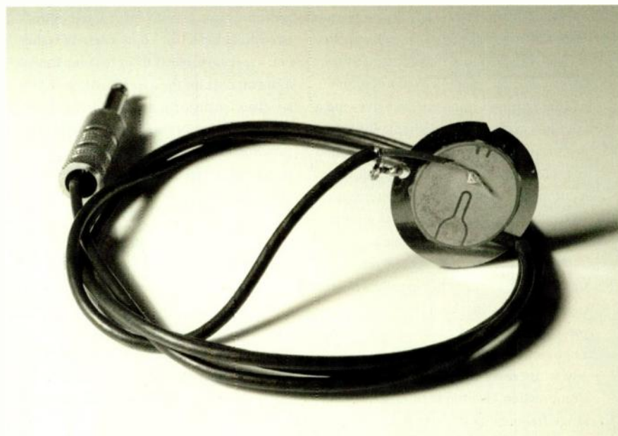
FIG. 2: Harness your DIY powers and build your own contact mic to explore unusual sounds. Piezo discs are inexpensive when purchased online. All you need is a 2-conductor cable, solder, and a soldering iron. This homemade contact mic took only a few minutes to assemble.
