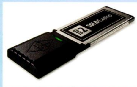
FIG. A: The UAD-2 Solo/Laptop card allows you to use Universal Audio's UAD plug-ins on your laptop.
