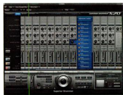
FIG. 2: Superior Drummer's Mixer lets you set how much each drum's bleed will be heard in individual mics.
