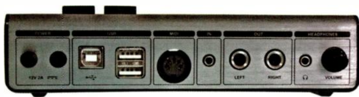
FIG. 2: The V-Machine's tidy rear panel sports plenty of USB connectors alongside unbalanced outputs and a stereo 1/8-inch input jack.
