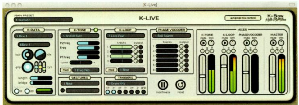
FIG. 1: In this screen from the K-Bow application, a player can monitor the output of the various sensors and control the DSPs, looping sequencer, vocoder, and volume levels of each module.
