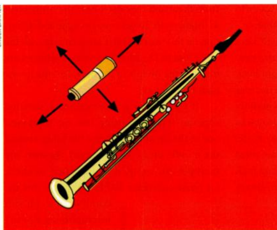
FIG. 2: Moving the microphone toward the mouthpiece accentuates the highs; toward the bell increases the cutting power and honk. Close-miking emphasizes warmth and high- and low-frequency details, while distance-miking yields a more natural sound.
