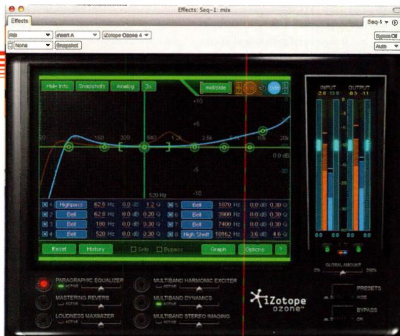
FIG. 1: Ozone's Paragrophic Equalizer module in M-S mode shows the EQ curve for the mid and side channels in orange and blue, respectively. Note the analog-modeled highpass filters' overshoot. The I/O meters are showing M-S levels here.
