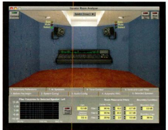
FIG. 2: Equator Room Analyzer automatically compensates for the room's primary modes and secondary reflections. It can save settings as presets to tailor the monitors' response to different circumstances.
