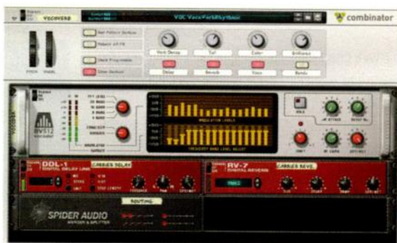
FIG. 1: In this Reason 4 Combinator, audio is routed through the DDL-1 and RV-7 to the Vocoder Carrier input. The dry signal is also merged to mono and used for the Modulator input.
