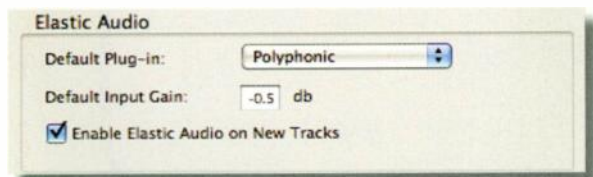
FIG. 2: Elastic Audio preferences let you choose which of the real-time plug-ins will be the default for new Elastic Audio-enabled tracks. This preference is linked to the plug-in chosen for preview in a browser.
