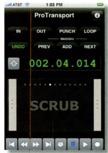
FIG. 6: Far Out Labs' ProTransport lets you turn your iPhone or iPod touch into a remote DAW-transport controller.
