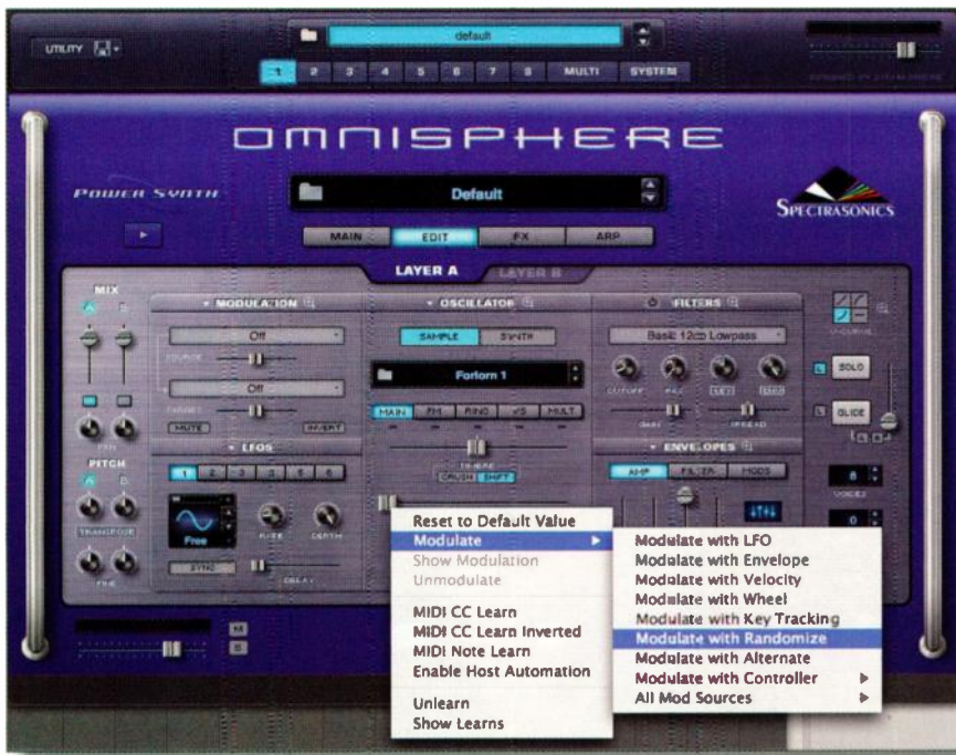
FIG. 4: Modulating the time within a sample at which it starts playing back can add life to the sound. This drop-down menu shows the variety of sources available in Spectrasonics Omnisphere for sample start modulation. (The Sample Start parameter itself is obscured by the drop-down menu in this illustration.)
