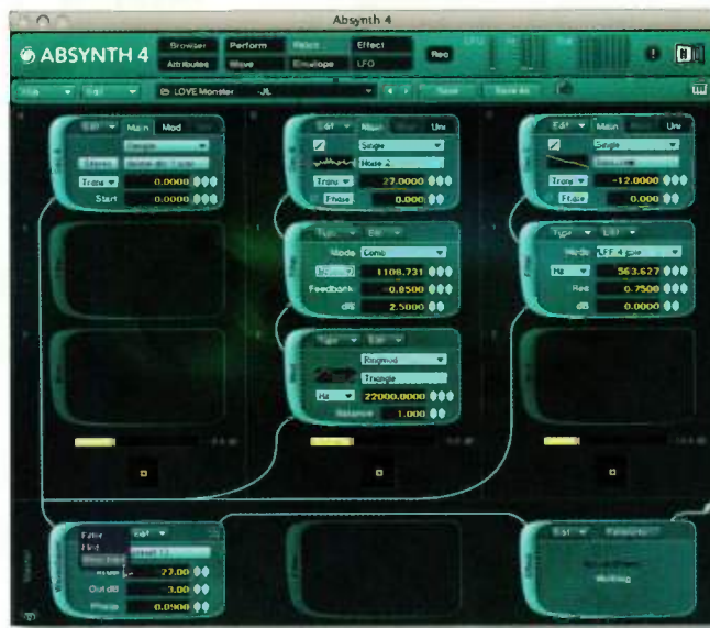
»» FIG. 1: In Native Instruments' Absynth 4, the signal path is user-definable. Each of the three oscillators feeds two modules that can be defined as a filter, modulator or waveshaper. There are two definable modules in the Master section, as well.
