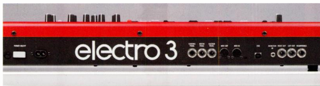
FIG. 3 In addition to MIDI In/Out and USB ports, the rear panel has two audio outputs, three control-pedal jacks and an input for routing an MP3 or CD player to the stereo headphone jack. The power connection uses an ungrounded two-prong cord.
