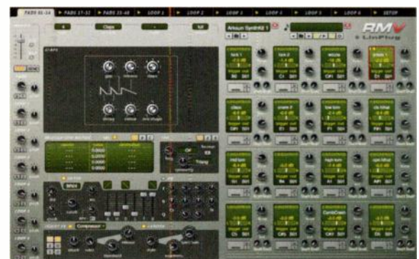
FIG. 2: On the left side of L nplug's RMV, I'm editing a snare drum pad using the Clap drum synthesizer. The top three knobs control the space between each clap, the release time and the number of claps. At the bottom-right of the left panel is the Varizer, which helps humanize the sound's playback.
