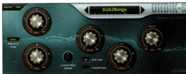
FIG. 1: The Uhbik-S frequency shifter's unusual options include offsetting the shift frequency and phase between stereo channels, and tempo-synched shift amounts.
