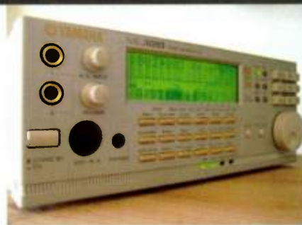
The Yamaha MU128's four audio inputs let me mix the output of two computers to stereo and capture it to a portable digital recorder.
