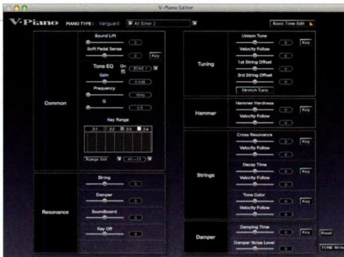
FIG. 3: All of the parameters that affect a Tone are available on the V-Piano Editor's Advanced Tone Edit screen, grouped by category.
