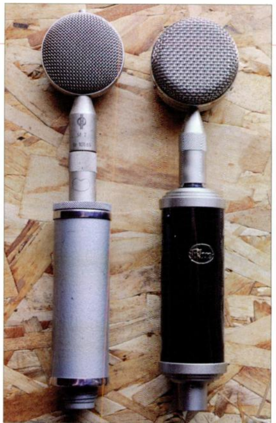
FIG. 1: The Bottle Rocket (this shows the Stage Two, right) and the Neumann CMV 563 are not only physically similar, but their mic capsules are interchangeable.
