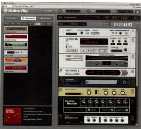
FIG. 3: In Native Instruments' Guitar Rig 3, you drag components from the GUI's upper-left to any positions in the rack on the right to establish their order in the signal chain.
