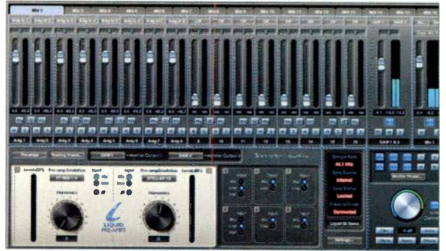
FIG. 3: A software-controlled, DSP-based mixer on the Saffire allows any 18 channels to be routed to any of 16 output channels with zero latency. It can also fold two channels back to the DAW.
