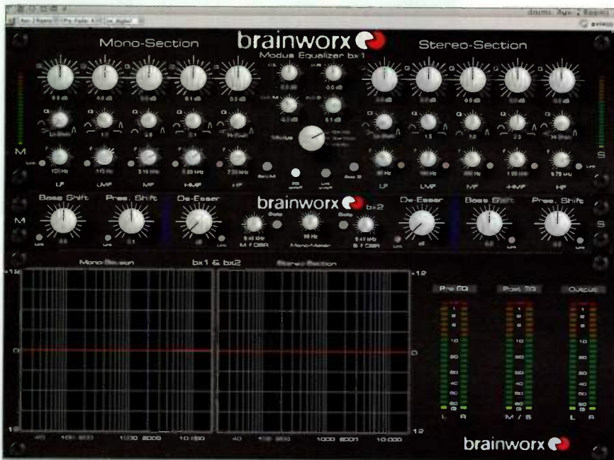
FIG. 4: In addition to conventional M/S equalization facilities, the Brainworx bx_digital plug-in provides a one-knob solution for centering bass frequencies in the stereo field.
