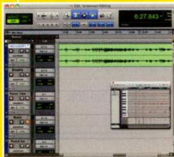
STEP 2: Set up additional tracks for breaths (lowered between -12 and -16 dB), room tone, music and dialog replacement.
