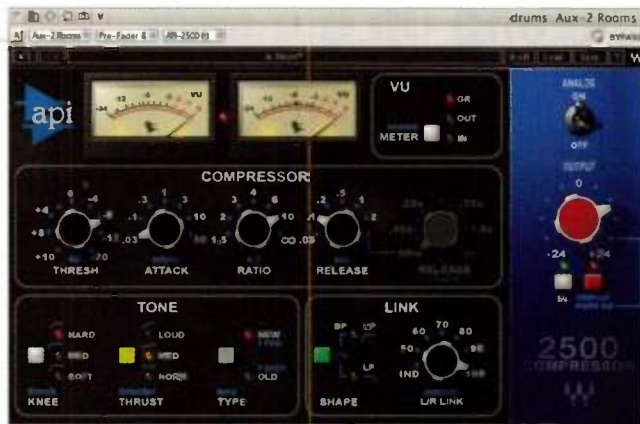
FIG. 3: The Waves API 2500 Compressor plug-in models the compression curve and character of the critically acclaimed API 2500 hardware bus compressor.
