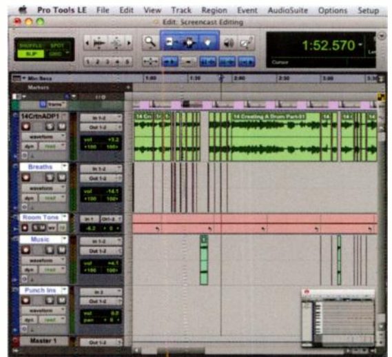
FIG. 1: Add polish to the mix by splitting the breaths and music from the dialog and placing them on their own tracks for individual processing.
