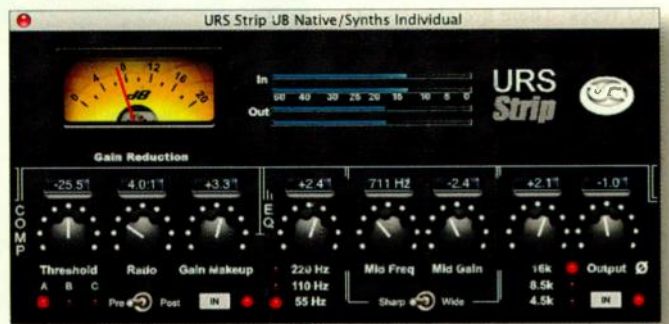
FIG. 4: URS Classic Console Strip specifically models a feed-forward, 1975 VCA gain-reduction amplifier with a transformer input.
