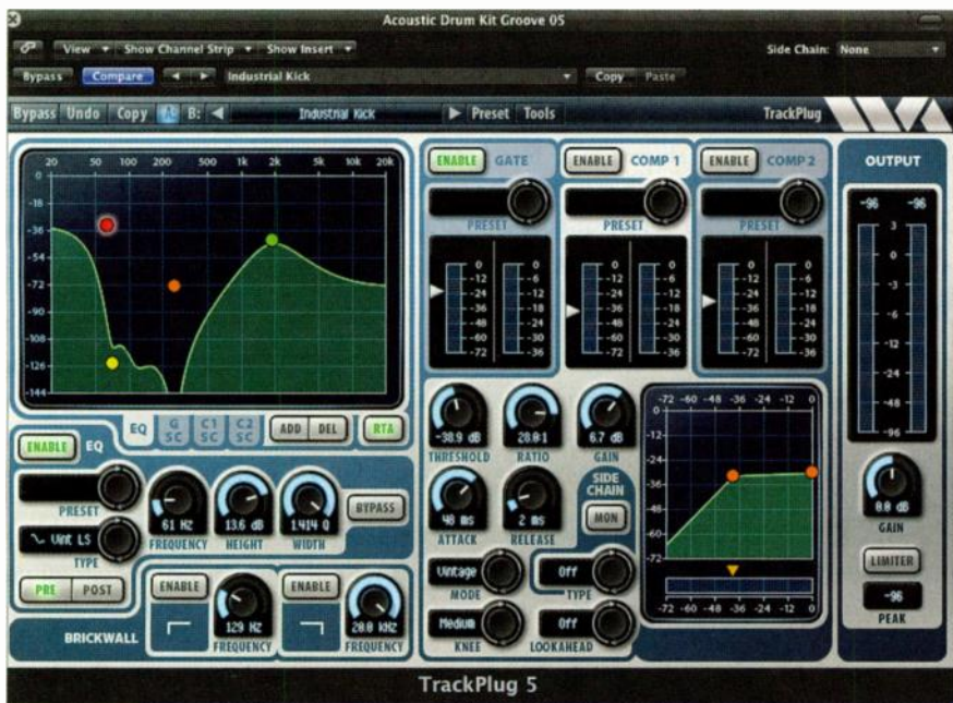
FIG. 5: Kitchen sink incoming! WaveArts TrackPlug 5 throws it all at you: gate, two compressors, 10-band EQ, 2-stage brickwall limiter and more.
