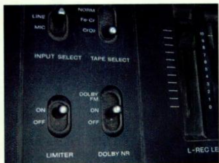
FIG. 4: Not only do old consumer cassette decks often have built-in limiters, but many times they also have an onboard noise-reduction circuit. After recording through it, try disabling the circuit for playback and you'll get an interesting exciter-style compression.
