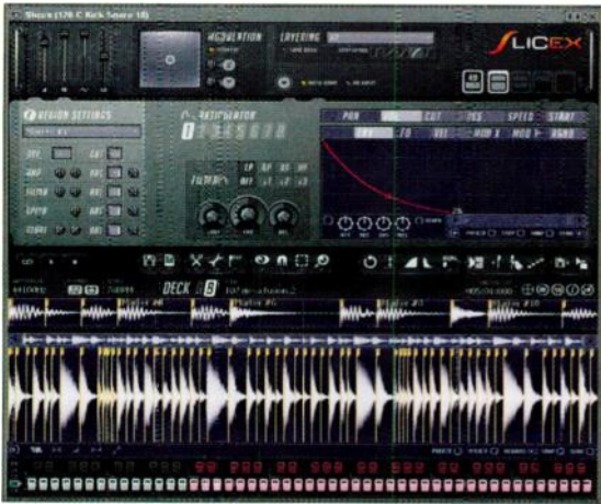
FIG. 2: FL's built-in Slicex instrument can slice loops, crossfade between two loops, send slices to separate mixer channels and process individual slices using as many as eight independent Articulators. Each Articulator has its own filter, LFO, envelopes and so on.
