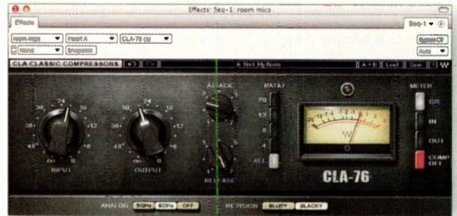
FIG. 2: CLA-76 offers two modes of operation that model different revisions of the classic 1176 FET compressor. The GUI for Blacky mode is shown here.
