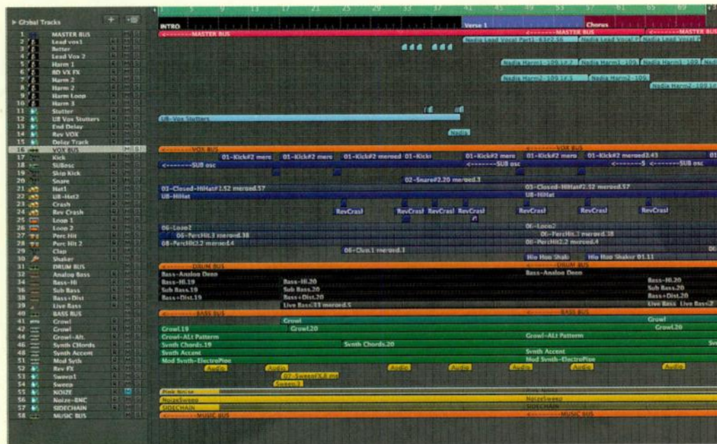
FIG. 4: Organization is the key. Here, all the tracks are arranged and color-coded with mix subgroups (in orange).
