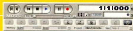
STEP 6: Slave your older DAW to external sync and press the Play or Record button to ready it for respective playback or recording in synchronism with the DAW in your newer computer.
