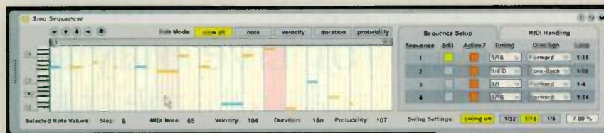
FIG. B: The new four-track Step Sequencer can produce complex patterns. Each track is monophonic and limited to 16 steps. Step length is programmed in the drop-down menus at right.
