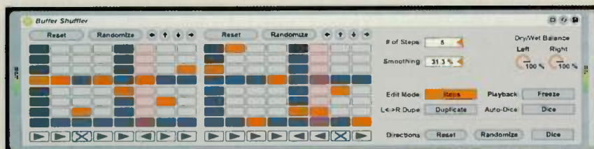
FIG. A: Buffer Shuffler slices and dices an audio loop. The orange spots on the grids show which slice will be played on which beat in the left and right channels (separately). The buttons at the bottom can reverse or mute any slice.
