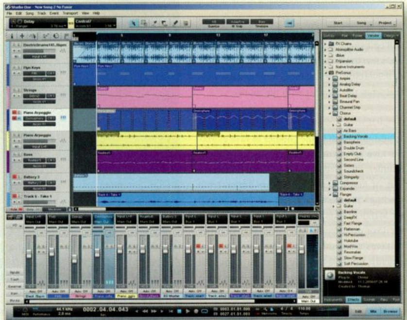
FIG. 1: The computer's F-keys open and hide the mixer and browser panels in PreSonus Studio One Pro. Note the fade-in on the first drum loop (upper left). Buttons are clearly labeled.
