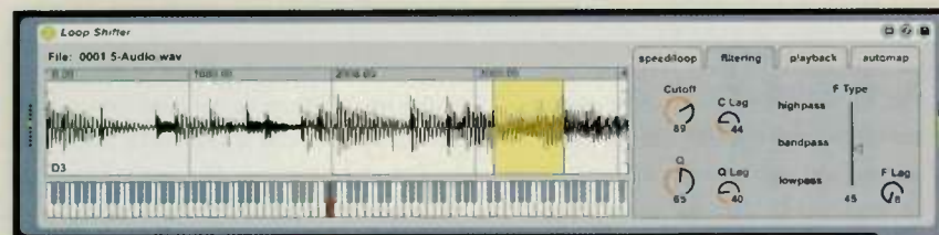
FIG. C: Loop Shifter produces its own signal rather than processing audio. After loading a loop, you can program each MIDI key to loop a separate section of the audio. Filtering, pitch and transition are separately programmable per key.
