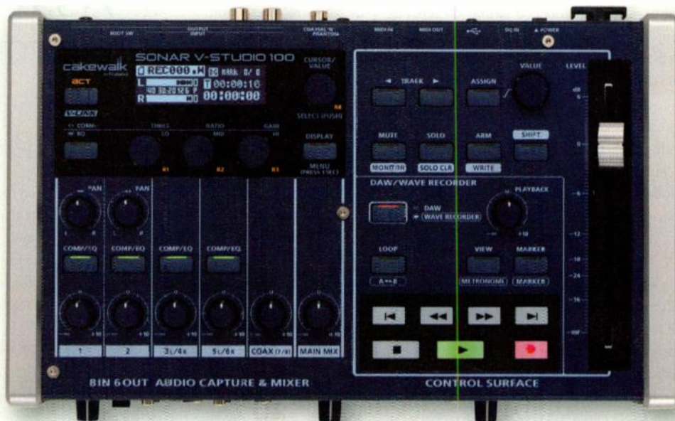
FIG. 1: The VS-100's relatively small topside area belies its ample capabilities. You can access many assignable features through a single-page menu and cursor system.
