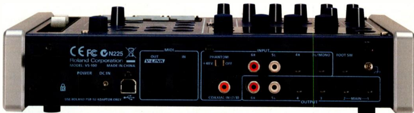
FIG. 3: A footswitch, additional inputs, MIDI I/O, USB, and a phantom-power switch adorn the rear panel. In addition to stereo Main-Mix outputs, you get individual outputs for channels 3 through 6.
