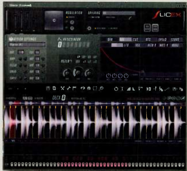
FIG. A: Slicex carves up sampled beats and lets you process each slice as needed. After adding or deleting slice markers, remember to click the Dump Score to Piano Roll button. You can control each of the six parameters listed above the envelope edit window (pan, volume, and so on) using any of the six functions in the second row (envelope, LFO, and so on).
