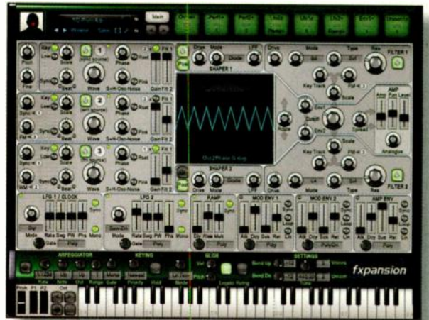
FIG. 2: FXpansion's DCAM Synth Squad bundles three diverse synths with a fourth that hosts all three. Cypher (pictured) specializes in analog modeling and audio-rate modulation synthesis.
