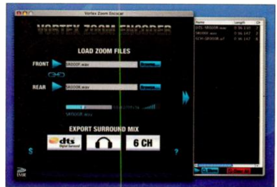
FIG. 1: Vortex Zoom Encoder (Mac/Win) converts a pair of stereo WAVs into standard surround files you can burn to disc or share online.
