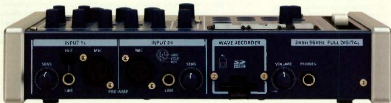
FIG. 2: Inputs 1 and 2 offer XLR or balanced 1/4-inch jacks. A front panel switch lets you change the first channel to high impedance.
