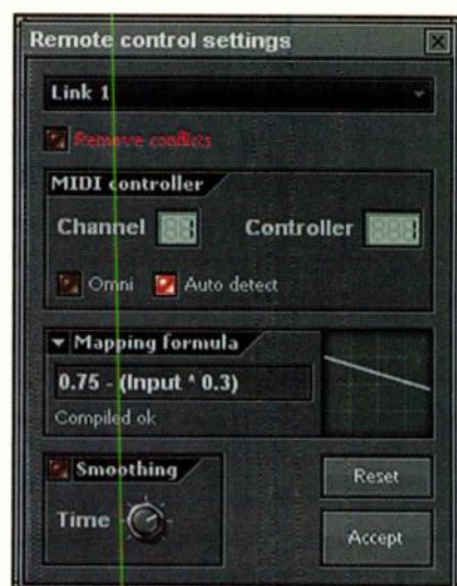
FIG. 3: In the Remote Control Settings box for a knob or fader, you can select a MIDI Control change input, write a formula to map the input values (range 0-1) to output (also 0-1), and more. A given knob or fader can respond to several different MIDI messages—just select New Link in the dropdown menu at the top.
