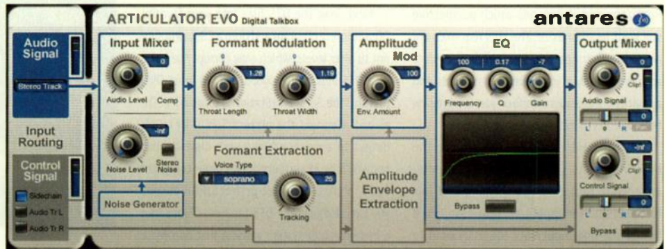
FIG. 1: Antares Articulator is ideal for vocoding diverse material with scat vocal snippets. Use the formant controls in the middle to tweak the vocal analysis.
