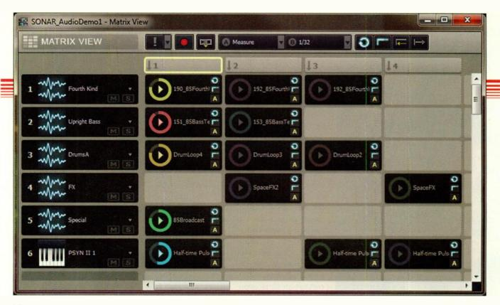
🔊 FIG. 1: The Matrix view, modeled after Cakewalk's Project5, allows for nonlinear cell-based triggering of audio and MIDI loops.
