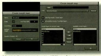
FIG. 2: To use the spectral-morphing AET Filter, you first analyze zone groups to create morph layers (left) and then arrange layers into morph maps (right).
