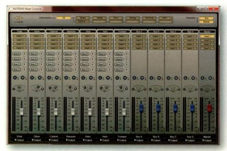
3-3- FIG. 2: Each channel in the Notion mixer has a level fader, pan pot, and mute and solo buttons. Each channel has four sends, one for each of the mixer's four aux buses, and can have up to four insert effects.
