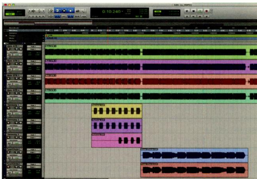
FIG. 1: A section of a song showing various layered guitar parts: a quadrupled main guitar, three harmonized guitars, and doubled power chords at the bottom.
