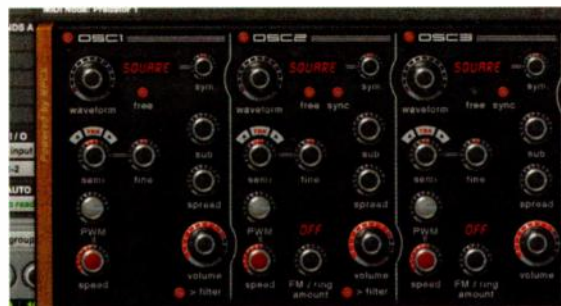
FIG. 2: Most synths use multiple oscillators to generate sound. By activating more than one, and adjusting parameters such as the waveform and pitch of each oscillator, you can get some really thick layers.
