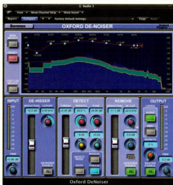
FIG. 2: DeNoiser offers an unprecedented level of control. The red line at the top is the Noise Threshold Bias control, which, along with the Noise Reduction Bias, gives you the ability to graphically fine-tune the noise profile.
