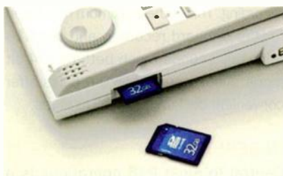
FIG. 3: The R16 stores up to 32GB of data on standard SDHC cards.
