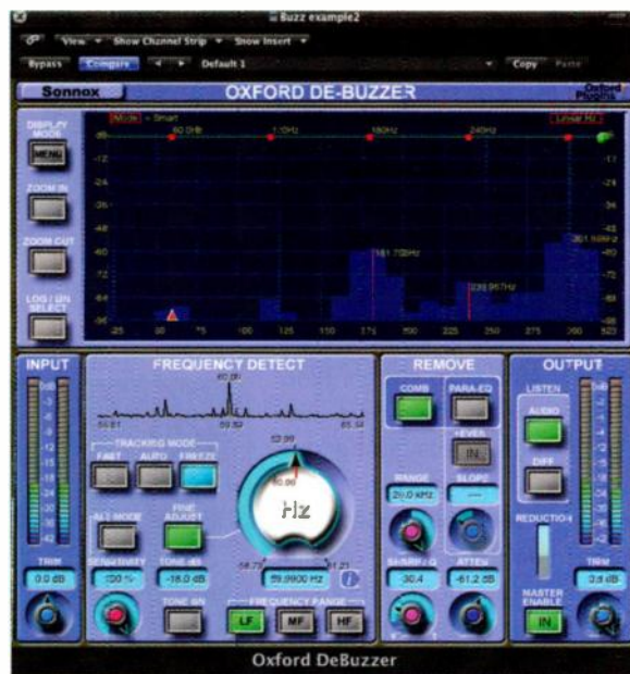
FIG. 3: DeBuzzer, like the other Restore plugs, offers a wide range of controls. The large white knob in the middle is for setting the fundamental frequency of a buzz or hum.
