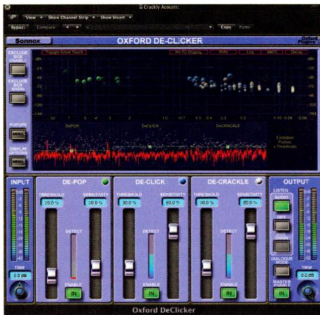
FIG. 1: DeClicker detects clicks, pops, and crackles and shows them as different color puffs in a screen called the Events Graph.
