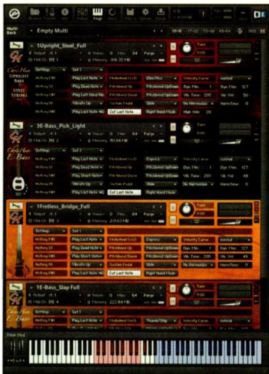
FIG. 1: Best Service Chris Hein Bass affords control over a large number of sonic artifacts. The notes highlighted in pink on the virtual keyboard are keyswitches used to activate different articulations.
