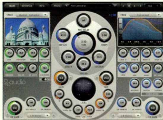
FIG. 1: This modified version of Aether's 150 Cathedral preset uses a mostly serial LR to ER signal path as indicated by the Cascade knob and switch settings.
