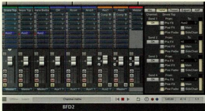
FIG. 4: The three ambience channels are sub-grouped to aux 1. Sidechain sends from the snare channels and the output of aux 1 feed the aux 2 channel.
