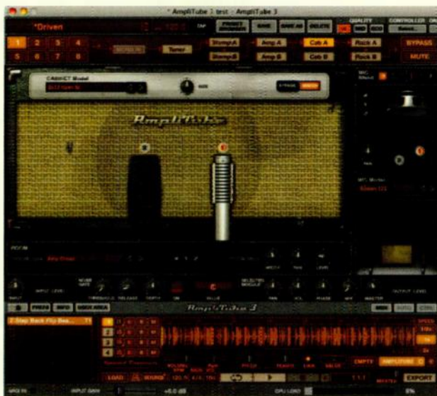
FIG 1: AmpliTube 3 features numerous improvements in a variety of areas. The most significant may be the revamped cabinet section, which lets you use two virtual mics, position them horizontally and back and forth from the cabinet, and pan their signals if desired.
