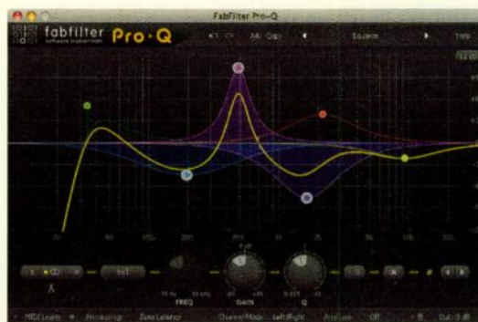
FabFilter Pro-Q offers mono, dual-mono, stereo, and mid-side equalization in an uncluttered GUI.
