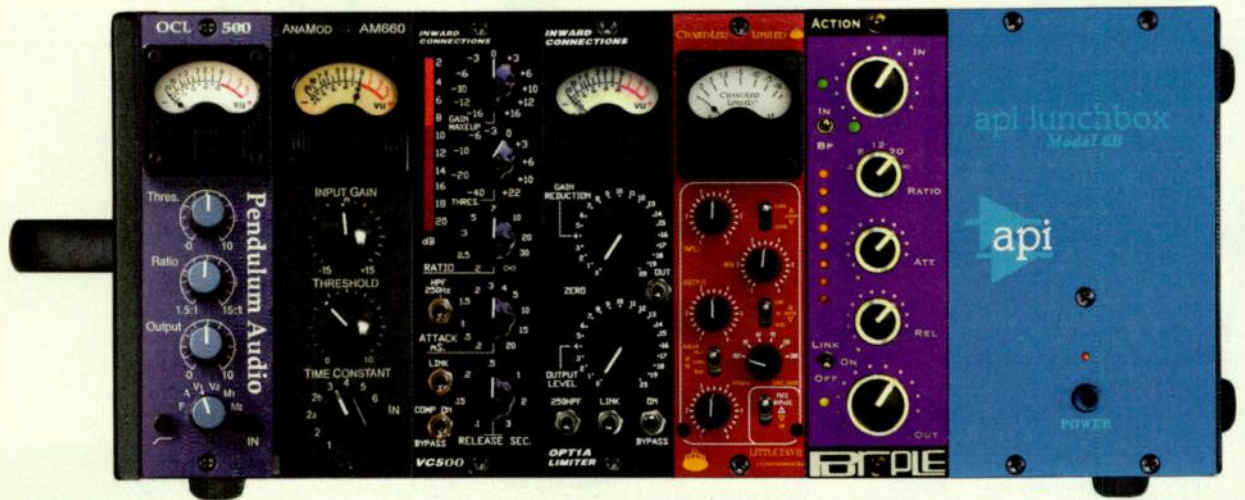
API's six-slot Lunchbox housing sparked a movement toward using 500 Series-format modules as outboard processors. Shown here are the six modules tested this month (from left): Pendulum Audio OCL-500, AnaMod AM660, Inward Connections VC500 and OPT1A, Chandler Limited Little Devil, and Purple Audio Action.
