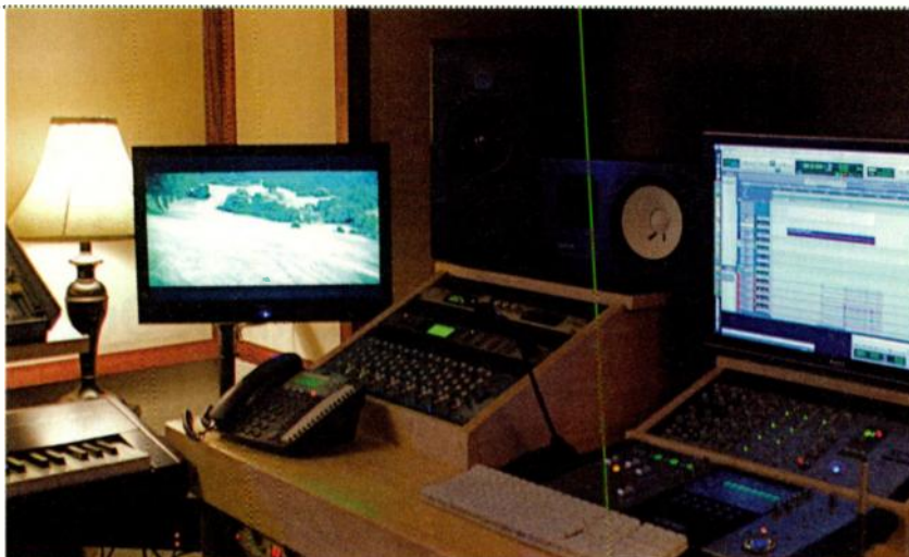
At Soundcake in Chicago, Brando Triantafyllou uses an Avid Pro Tools HD4 rig and Euphonix MC Control in HUI mode to compose and mix.
