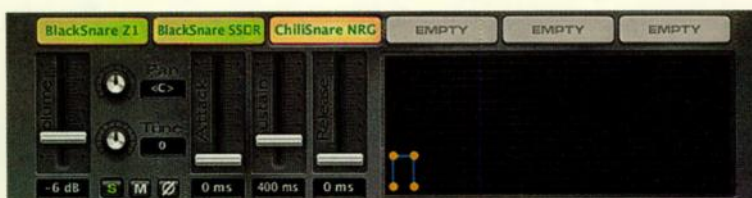
FIG. 3: The ASR envelope (bottom-center of figure) of a Trigger instrument derived from room mics can be edited to create gated-reverb effects.
