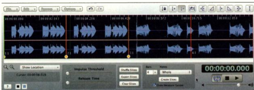
FIG. 2: I've used AudioFinder's Sample Tool to slice an 8-bar bass stem into 2-bar slices. The red gridlines are at 2-bar intervals, and the yellow-handled markers indicate the slice points. The slice marker at 4.1 was deleted to preserve the 4-bar phrase.
