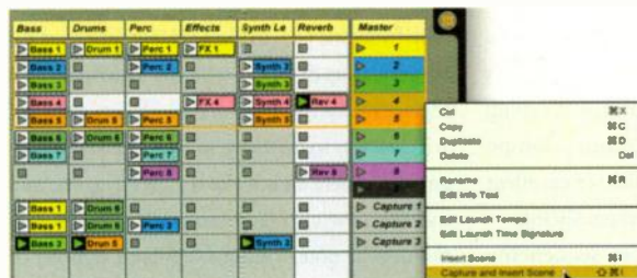
FIG. 3: Slices from a 6-part arrangement in Ableton Live occupy Session view Clip slots (top). Three Scenes are captured at the bottom, and the Rev 4 clip is playing along with the third captured Scene.
