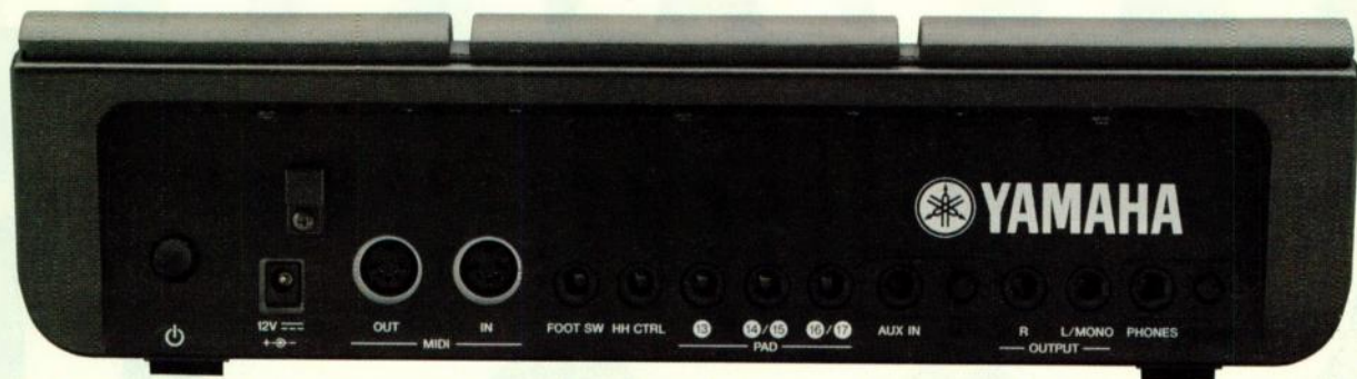
FIG. 2: Rear panel I/O includes MIDI In/Out, five inputs for control pedals and external pads, a 1/4-inch aux input, a pair of 1/4-inch outs and a headphone output.
