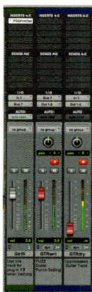
FIG. 1: The aux track (left) hosts my plug-in and routes it to the middle track. The right track records the unprocessed signal, which I've noted in the comments field at the bottom.
