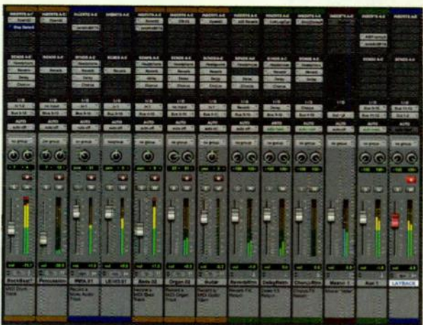
FIG. 6: You can print effects during a layback by using an aux track before the destination track.
