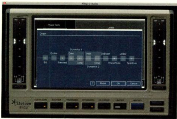
FIG. 2: The Graph window lets you rearrange the modules however you like, including setting up the two compressors in parallel or in series.
