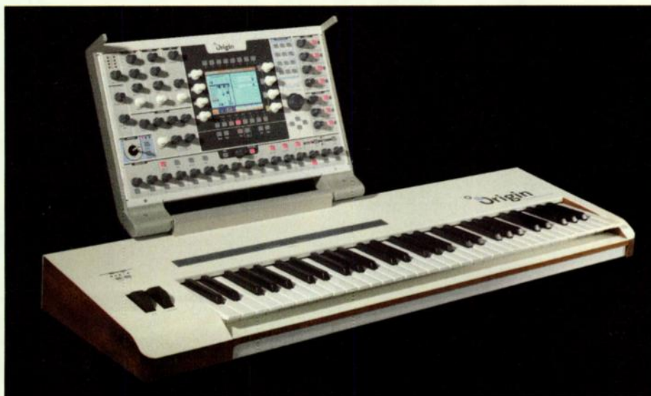
FIG. 1: The Origin Keyboard updates Arturia's first hardware synthesizer, the Origin, previously available only as a rackmountable tabletop module. Among other features, it adds a versatile ribbon controller and duophonic aftertouch.
