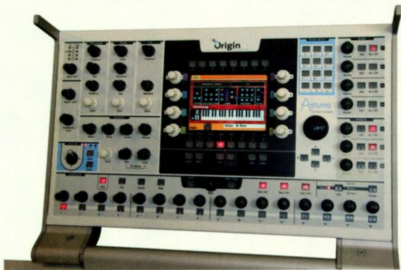
FIG. 2: The Origin Keyboard's flip-up control panel is identical to the original Origin and comprises 54 knobs, 81 buttons, a joystick, and a backlit color LCD.
