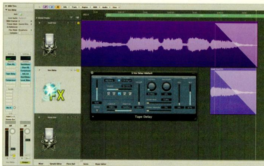
FIG. 1: When you want to delay a single word, copy it to a new track, insert a delay, and set its mix to 100-percent wet.
