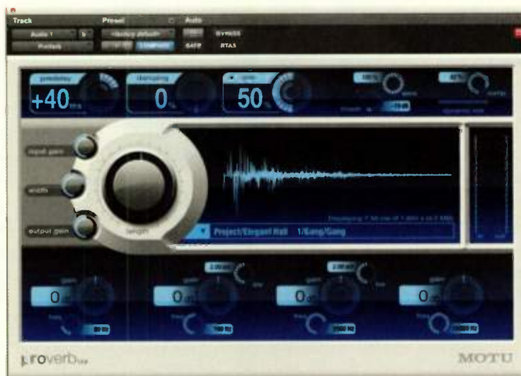
FIG. 3: ProVerb's dynamic mixing section is set to "duck" the level of the reverb within the plug-in's internal mix, based on the level of the dry signal.
