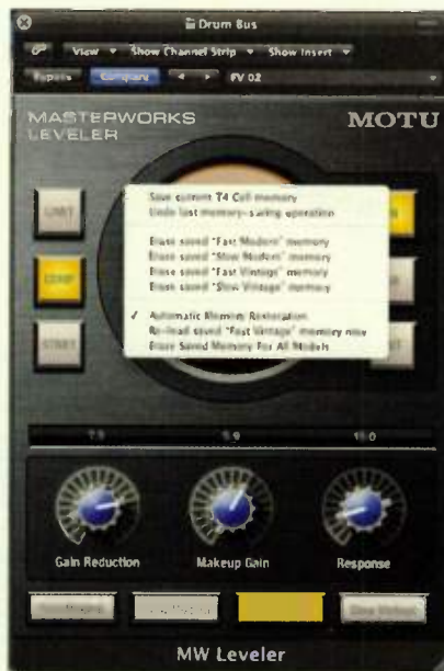
FIG. 2: Leveler's memory-management menu lets you save the “warm” state of the T4 cell after a waking stage where it's “primed” by the underlying program material that is played through it.
