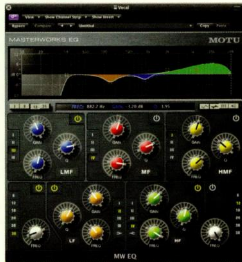
FIG. 1: The four different EQ filter styles are used on different bands of a MasterWorks EQ placed on a female lead vocal track, combining corrective precision with broadband sweetening.
