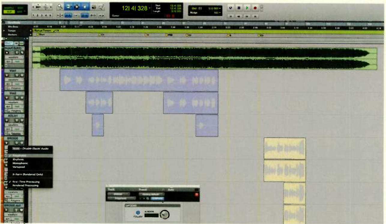
FIG. 1: Getting the vocal track—and any of the other tracks from the original version—time-stretched to your new tempo is an important, early step in a remix project. In this instance, the stretching is being done with Pro Tools' Elastic Time feature.
